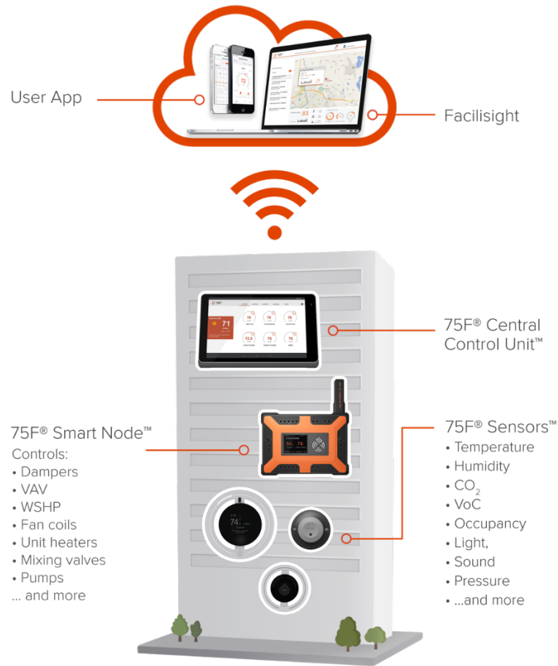
Figure 5. Example of a Central Controller Unit (source: 75F 1 )
