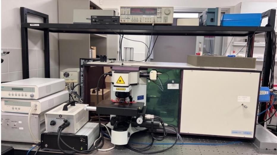
*Figure 2.3: Raman spectroscopy by Horiba's HP 800 spectrometer.*
