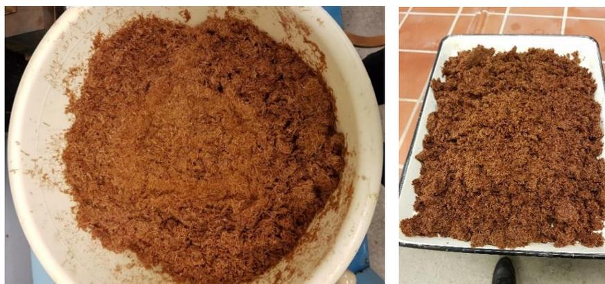
Figure 2.3 Modification by Silane (left), fully modified samples ready for drying (right)
