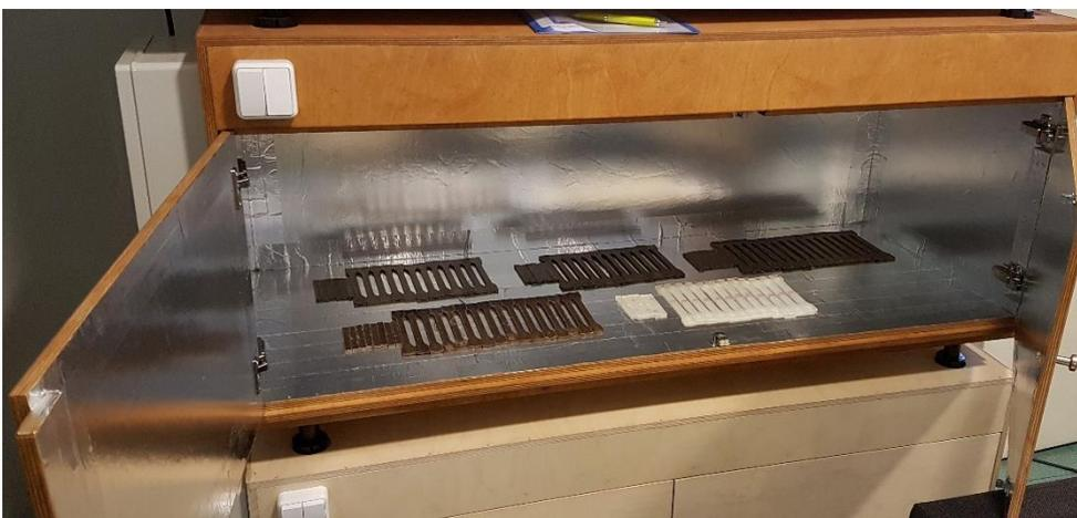
Figure 2.12 Specimens in the UV chamber ready for artificial weathering
