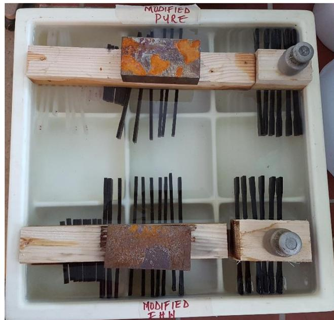
Figure 2.11 Specimens immersed in water for 28 days
