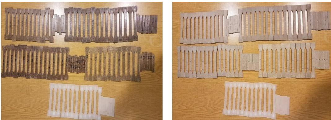
Figure 3.10 Neat PP and composites before (left) and after exposure (right) to UV radiation for 2016 h in the UV chamber
