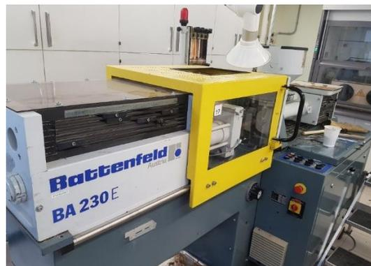
Figure 2.5 Battenfeld BA 230 E injection moulding machine
