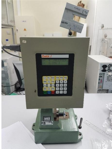
Figure 2.10 Zwick Charpy 5102 pendulum impact tester
