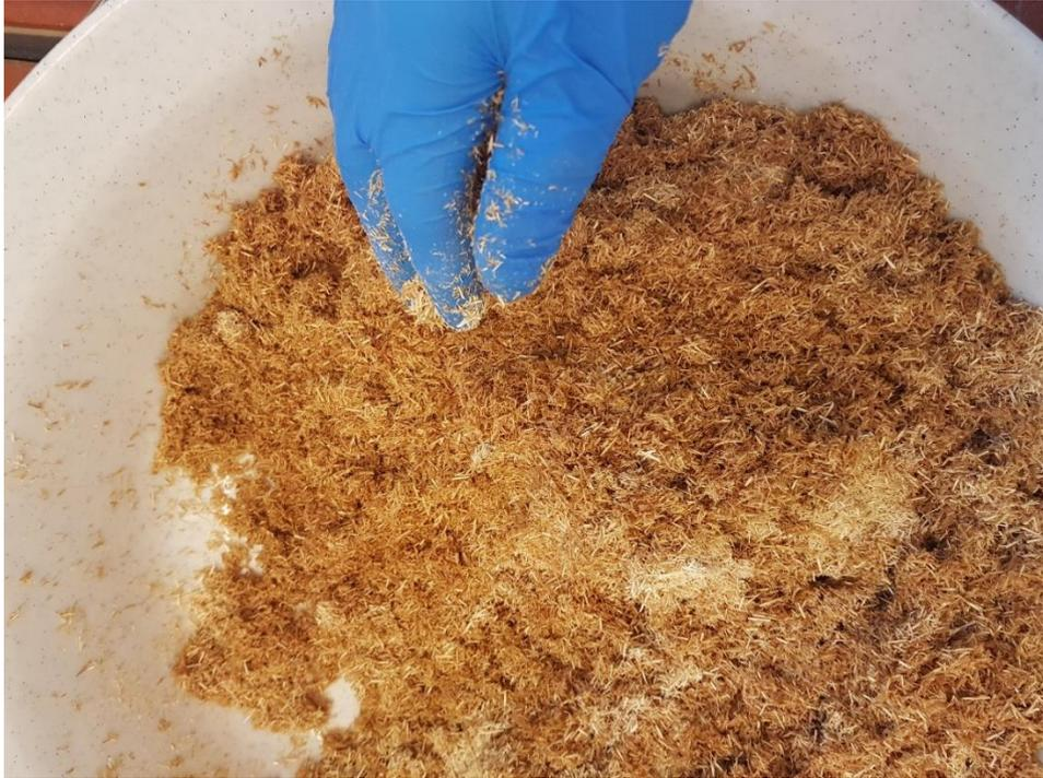
Figure 2.1 Modification of wood with NaOH
