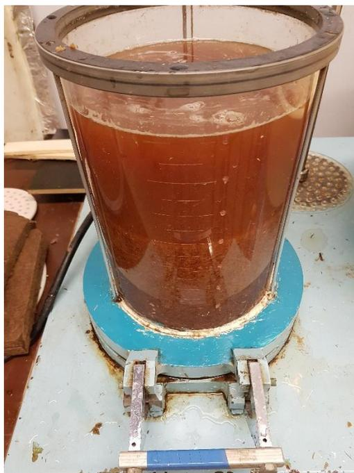
Figure 2.2 Rinsing of WF modified in NaOH using a vacuum
