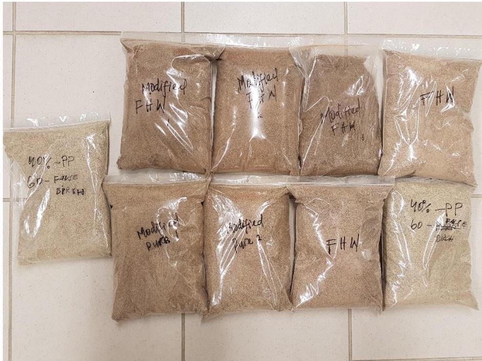
Figure 2.4 Compounded samples sealed in plastic bags awaiting injection moulding
