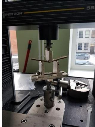
Figure 2.9 Flexural test of a specimen
