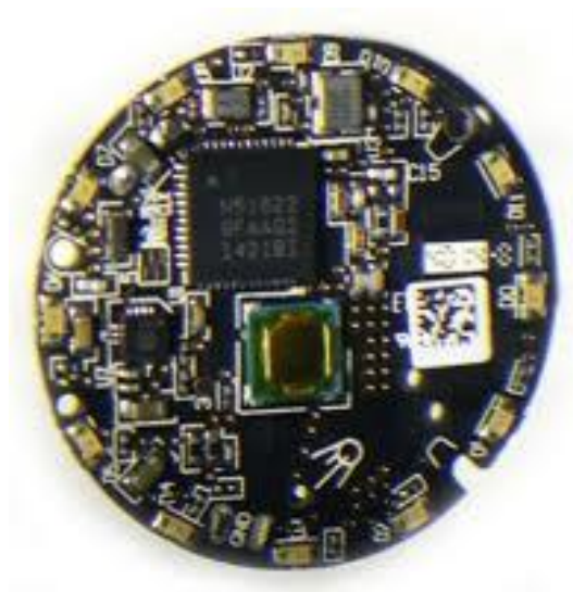
Figure 2 MisFit FLASH activity tracker board
