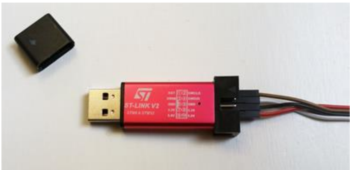
Figure 6 ST-Link v2 type programmer used for current thesis
