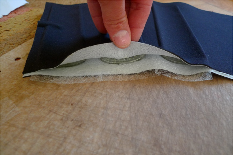
Picture 41 Thermo-adhesive material installed in-between the final opened edge to glue it together
