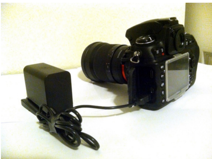
Picture 19 External battery connected to Nikon D700 through DC IN socket (Kingham, 2012)
