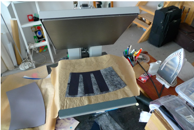
Picture 37 Manual thermo-transfer press with bottom layer of neoprene and thermo-adhesive material on it
