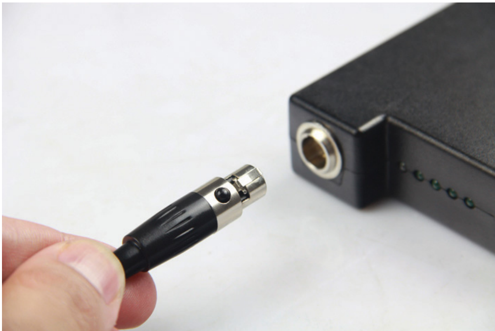
Picture 24 LanParte is using 3-pin xlr connector in their PB-600 external battery ( www.hdvideoshop.com , 2014)
