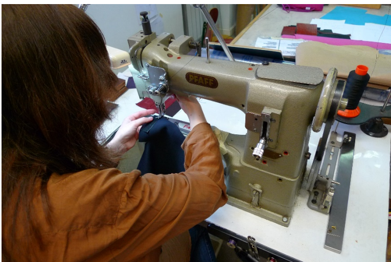
Picture 33 Sewing Velcro on the neoprene, using leather sewing machine
