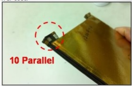
Picture 5 Prologium thin flexible Lithium-Ceramic battery cells connected in parallel (www.prologium.com, 2014)
