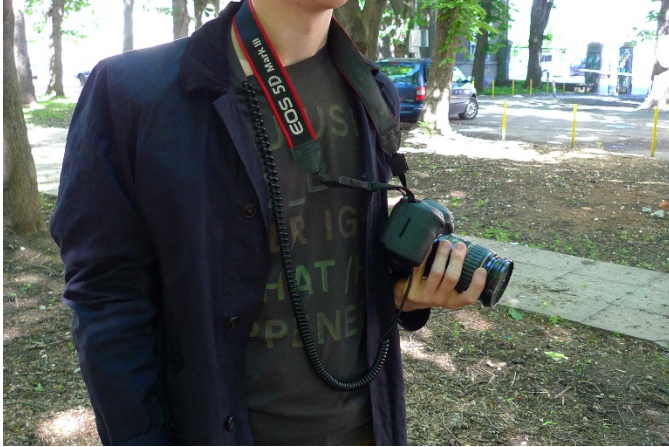
Picture 55 Spring-cable coming out from the collar
