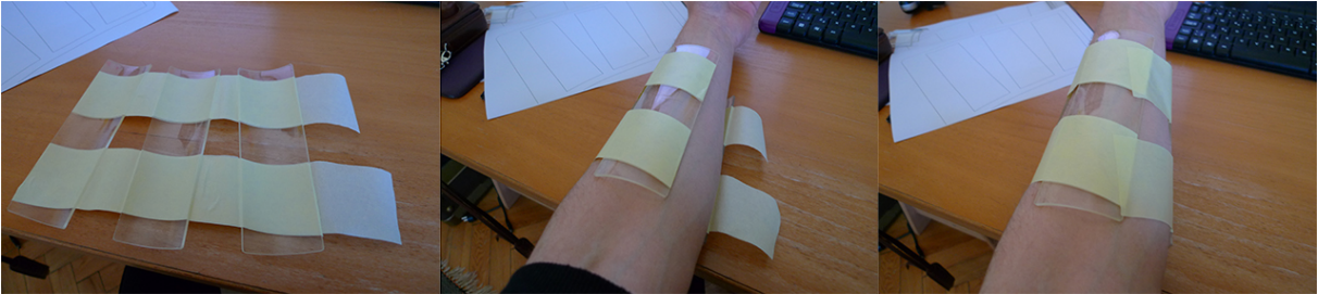
Picture 31 Mock-up for testing out different radiuses for Li-Po cells
