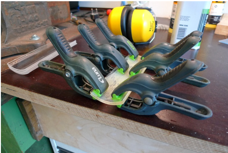
Picture 32 Gluing together two layers of Plexiglas to achieve right thickness
