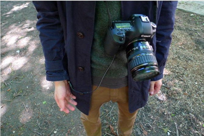
Picture 48 Battery Sleeve connected to the camera using short wire
