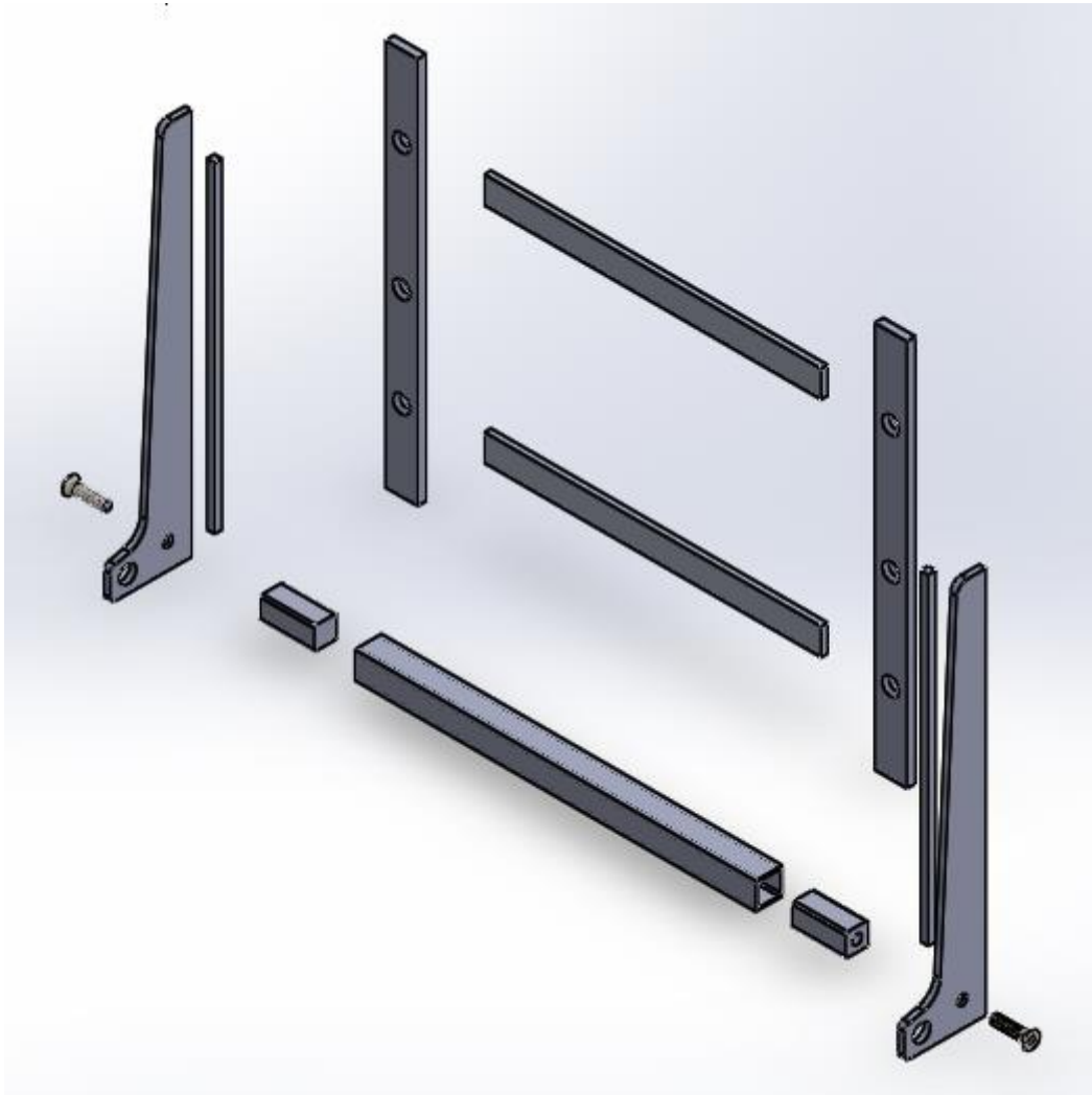
Figure 42 Exploded view of Improved Mount Structure
