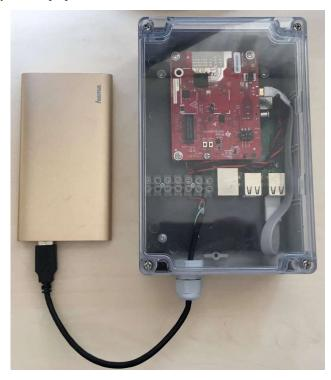
Figure 6. AWR1843BOOST and Raspberry Pi 3 B+ in box connected with power bank output 5 V, 2100 mA  $\,$
