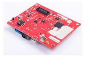
Figure 33. AWR1843BOOST AWR1843 single-chip 76 - GHz to 81 - GHz automotive radar sensor evaluation board image.
