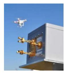
Figure 3. Photograph of the radar front end of the MuRPS.
