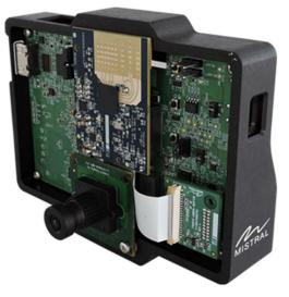
Figure 41. Sensor Fusion Kit
