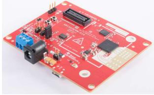
Figure 35. AWR1443BOOST AWR1443 single-chip 76-GHz to 81-GHz automotive radar sensor evaluation board image (angled view)
