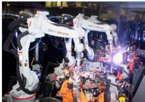
Figure 5. Welding robot in operation [6].
