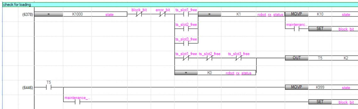
Figure 28. State 1000 in ladder diagram.
