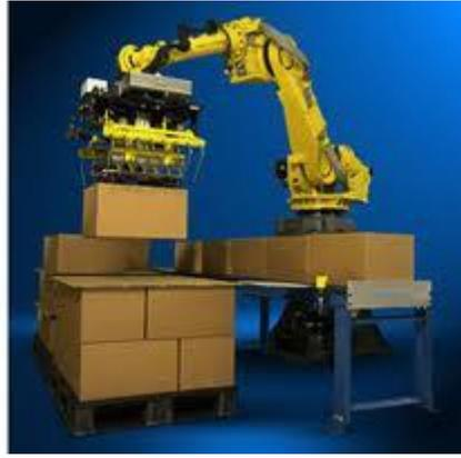
Figure 7. Palletizing robot in operation [6].
