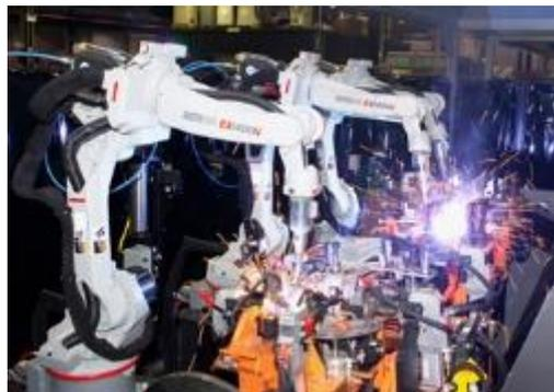
Figure 5. Welding robot in operation [6].
