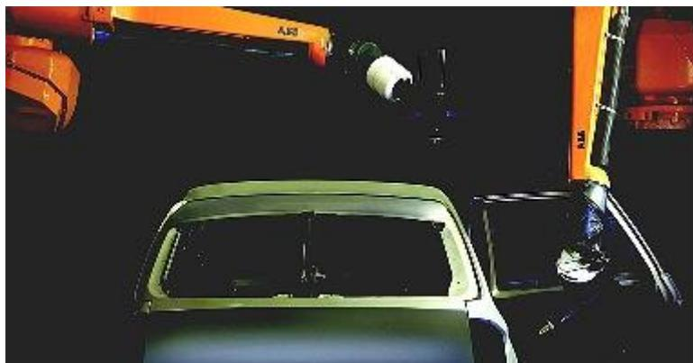
Figure 3. Painting robot in operation [6].
