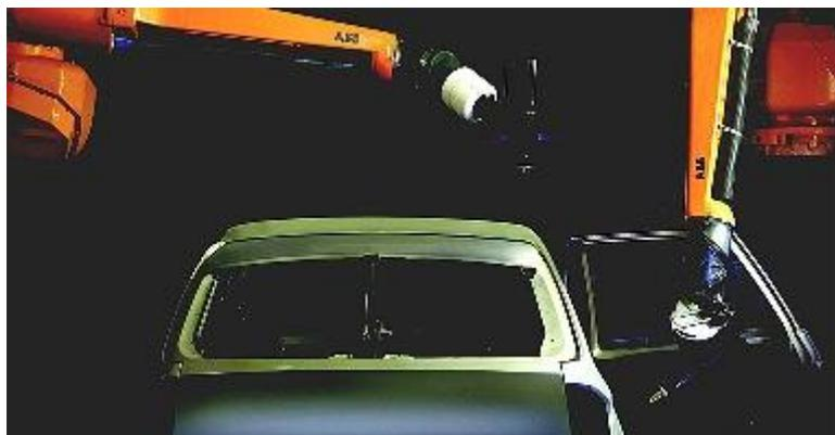
Figure 3. Painting robot in operation [6].
