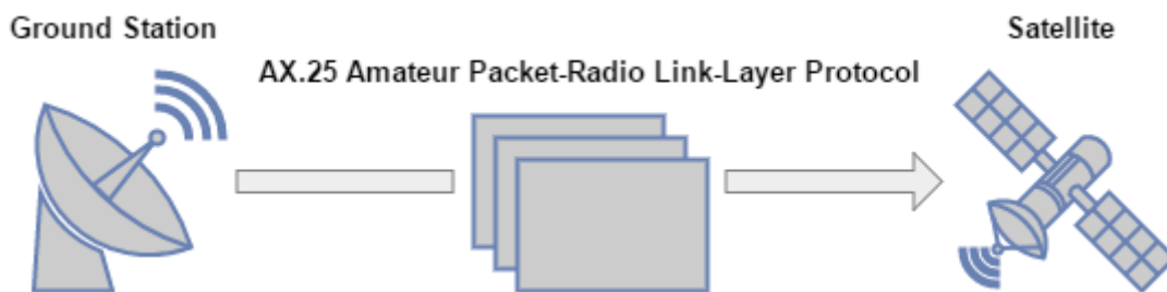
Figure 2. TTÜ-Mektory Student Satellite communication protocol.
