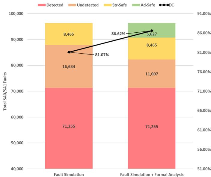
Figure 34: Combined Results in CPU [10]
