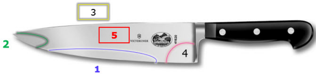
Figure 8 Functional Part of Blade
