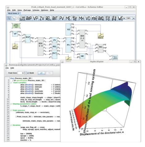
Figure 7.2: Simulation of a hydraulic-mechanical load-sensing system
