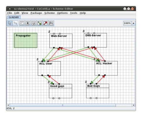
Figure 7.3: Visual specification of a response analysis problem in GrADAR package
