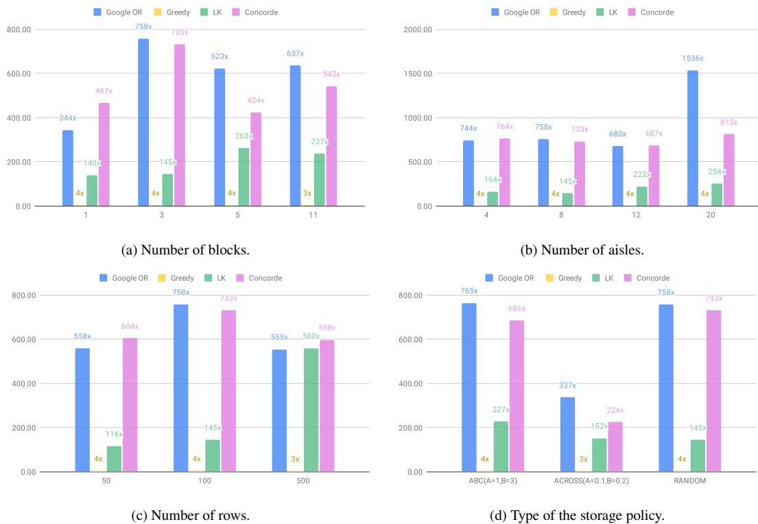
Figure 23. Bar Charts illustrating runtime decrease of the TSP solvers and algorithms when compared to 2-opt with different changing parameters.
