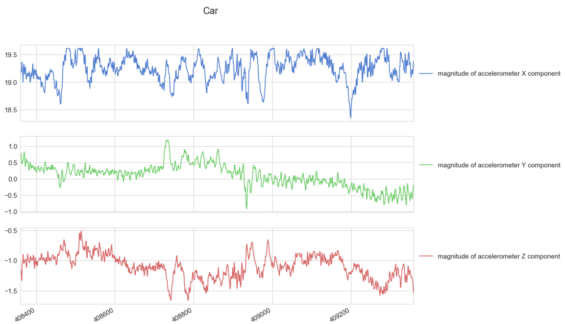
Figure 9 Car activity magnitudes of accelerometer components ( m/s^2 ) for \sim 6 s
