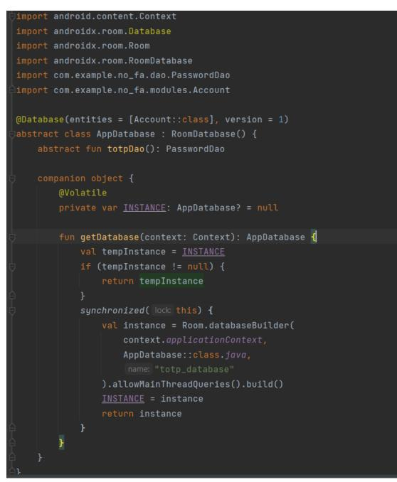
Figure 12: Android application database class implementation code
