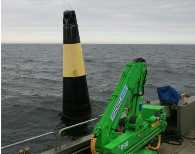
*Figure 3.8: Steel spar buoy [69]*
