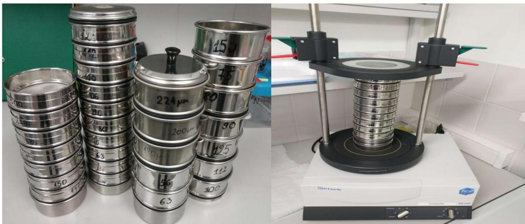
Figure 2.1 Scheme of sieving machine.
