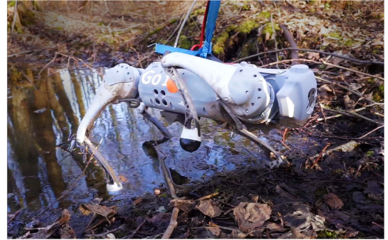
Fig. 1. The Unitree Go1 robot used in this research. The IMU is located at the center of the trunk, and each leg has three motors: one for the hip joint, one for the thigh joint, and one for the tibia joint. See also Fig. 2.
