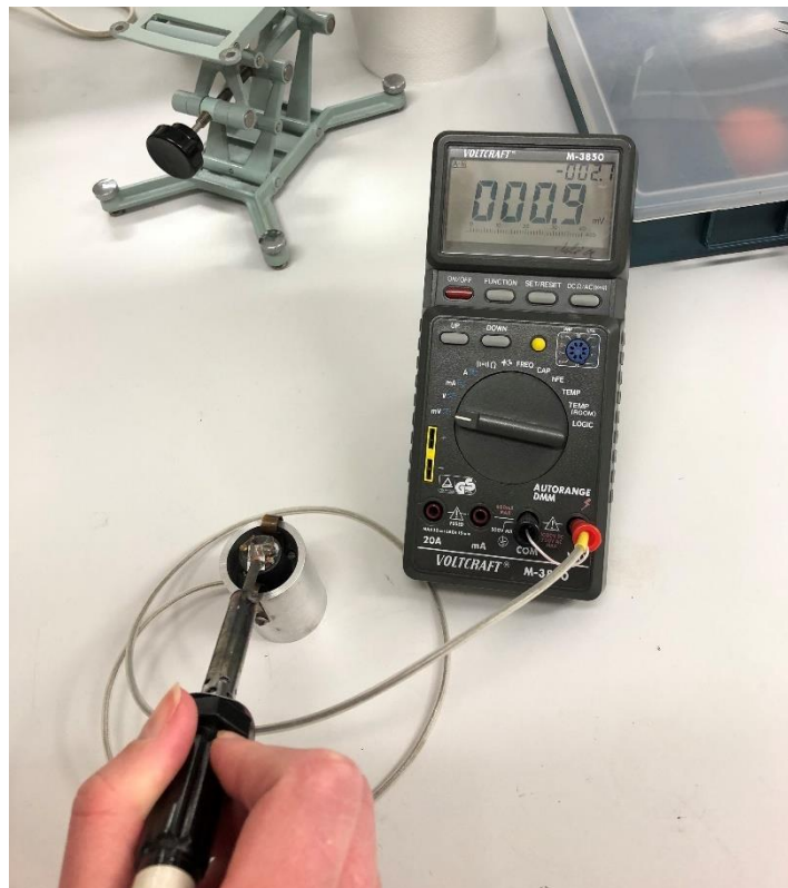
Figure 3.11. Hot probe experiment with pyrite powder crystal showing n -type conductivity
