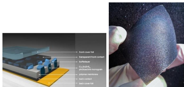
Fig. 1. Left schematic of MGL solar cell [8], right semi-finished MGL solar cell without encapsulant
