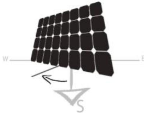
Figure 3.3 Azimuth angle of a solar panel [33].
