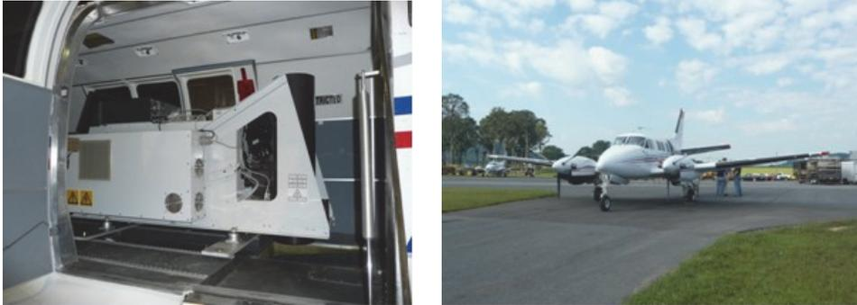
Figure 1. King Air 90 aircraft (right) certified for carrying FLS-AM (Airborne Multi-wavelengths) lidar (left)
