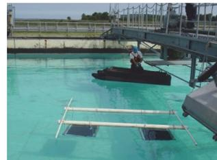
Figure 6. Installation of submerged targets with oil.
