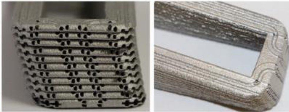
Figure 2.5 Additively manufactured aluminum alloy windings with a hollow structure for direct conductor water cooling [3].
