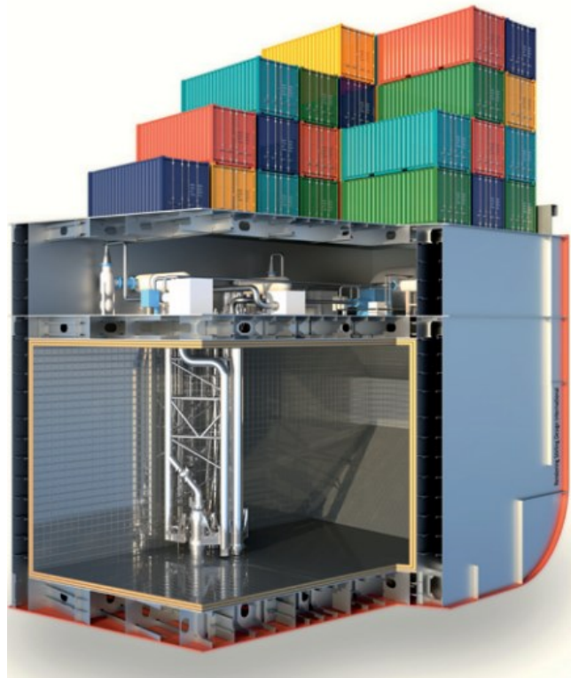
Figure 17: GTT membrane fuel tank
