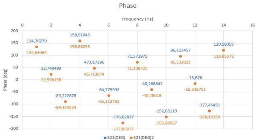
Figure 23. Stability of Phase. Huber + Suhner SF-526S cable No3.
