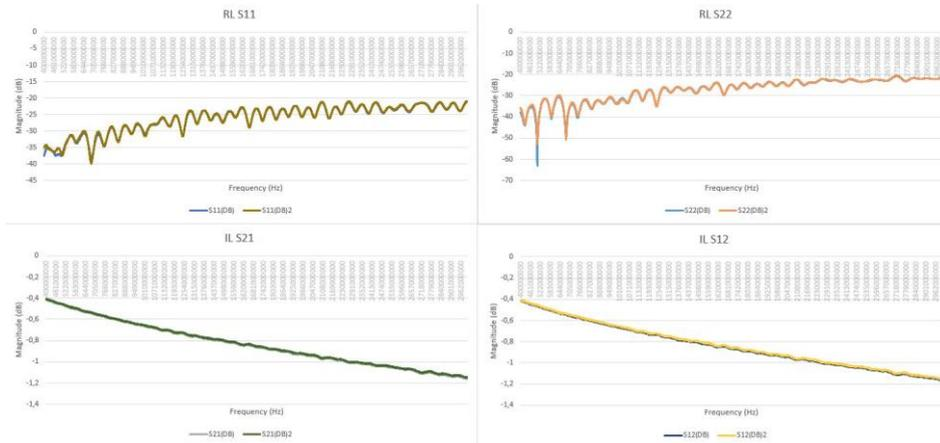
Figure 14. Stability of S-Parameters. Gore cable No3.
