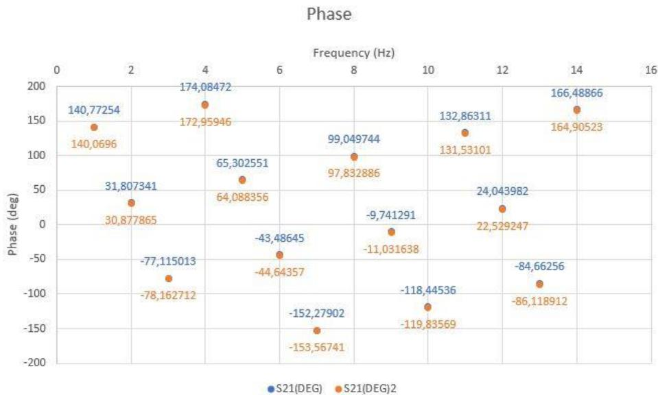
Figure 41. Stability of Phase. Rosenberger cable No4.
