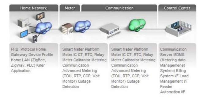
**Figure-3**: The Components of intelligent remote data collection for smart metering [15]. **Source**: http://www.moxa.com/solutions/AMI/index.htm
