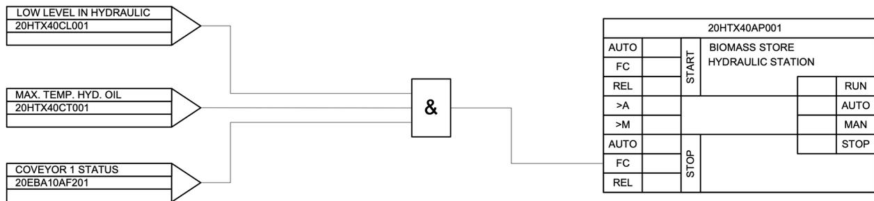
Figure 4.4: Hydraulic station interlocks
