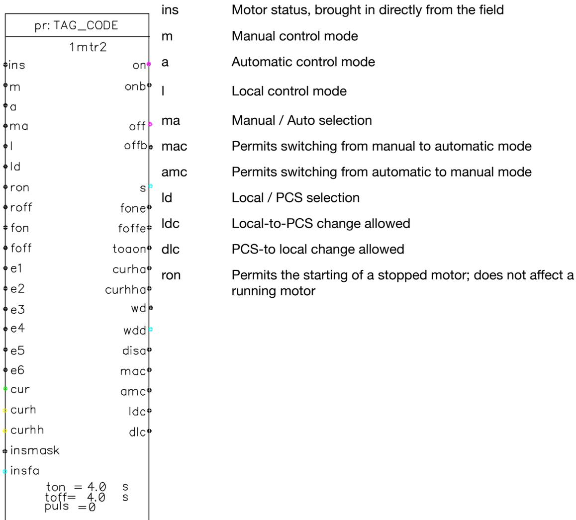
Figure 2.10: mtr2 block representation and basic inputs
