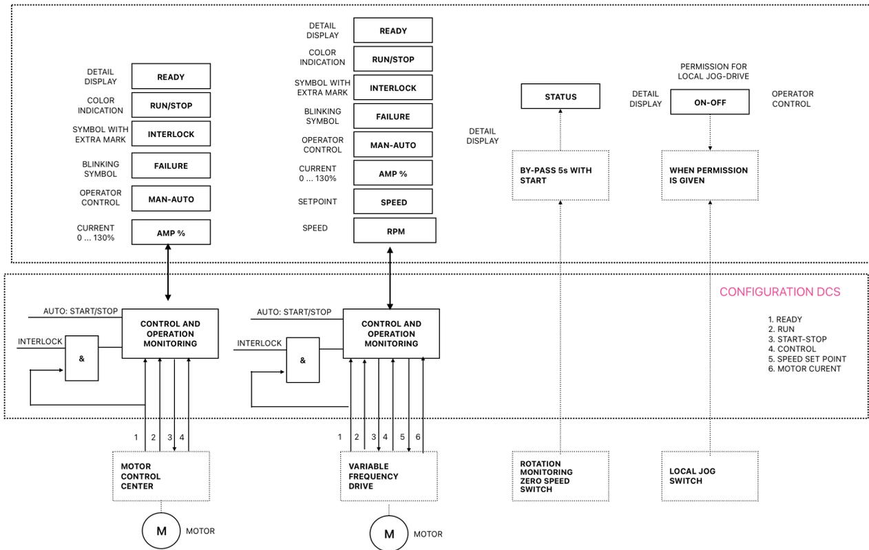
Figure 2.9: Schematic overview of DCS motor operations
