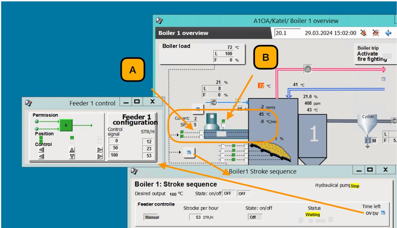
Figure 4.7: Feeders control operation display
