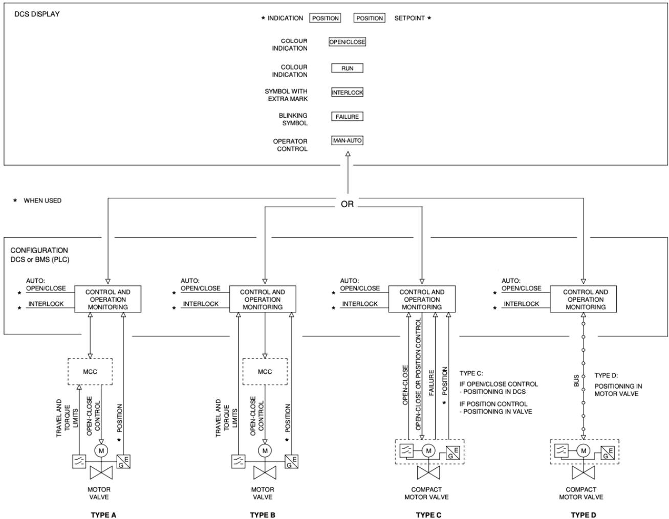
Figure 2.8: Schematic of DCS control and monitoring for motor-operated valves
