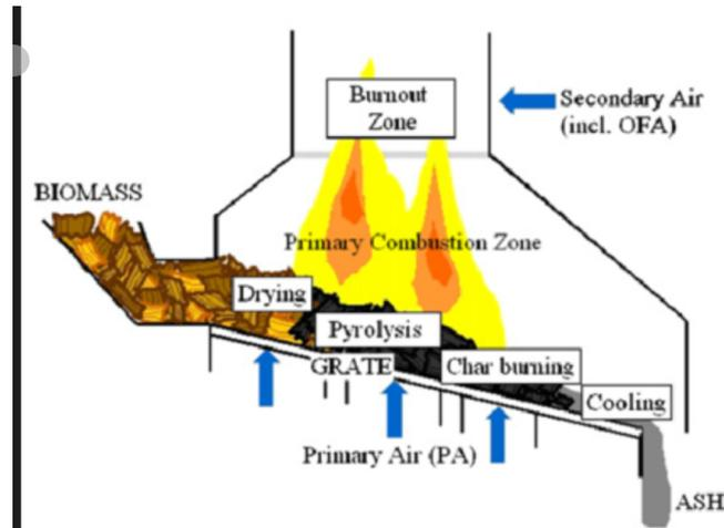
Figure 2.4: Grate combustion basic principle
