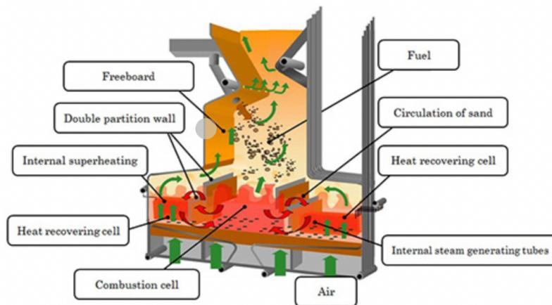
Figure 2.5: Schematic diagram of fluidized bed combustion process and components
