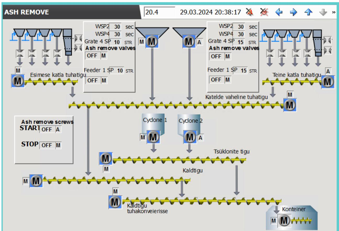
Figure 4.11: Ash remove operator display
