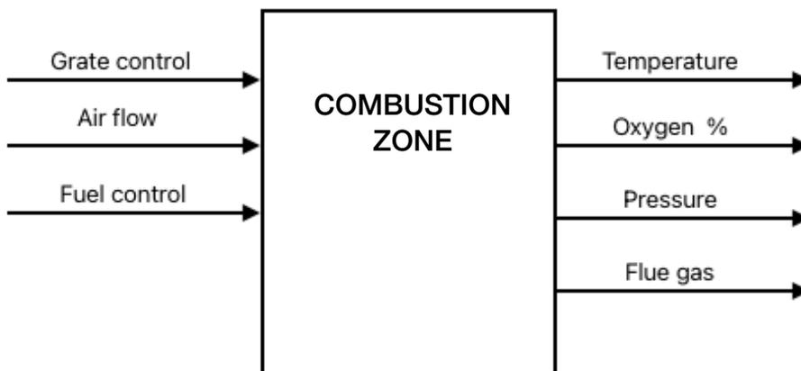
Figure 4.8: Basic Control Scheme for Biomass Combustion Process
