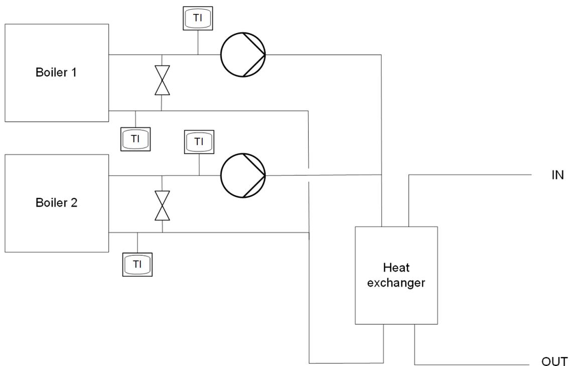
Figure 3.2: Principle water part diagram
