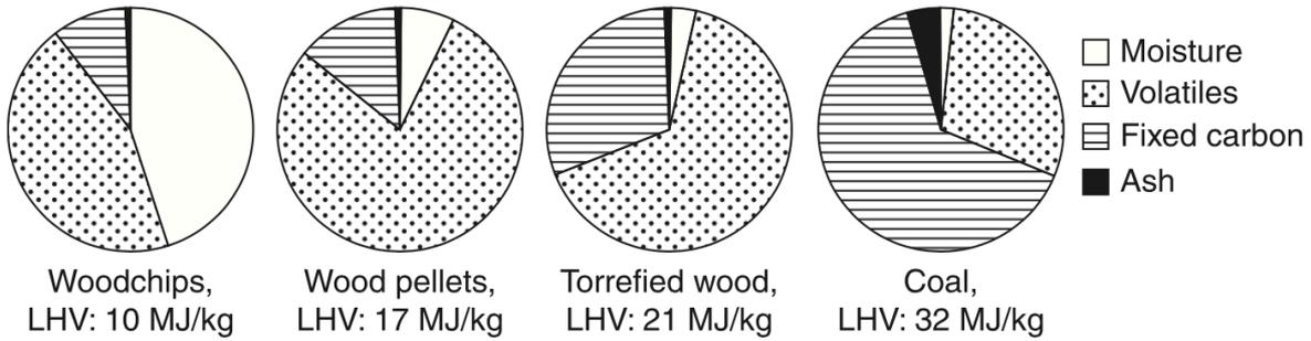
Figure 2.2: Comparative composition and energy content of biomass and coal
