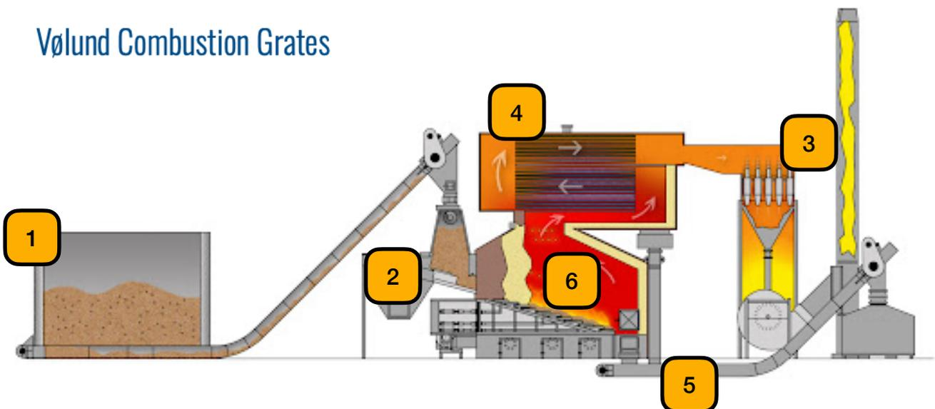
Figure 1.1: Schematic overview of grate combustion boiler system
