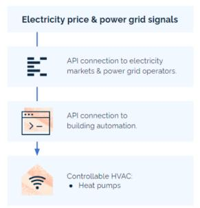
Figure 2.18 Kapacity.io API connection to building management system [51]
