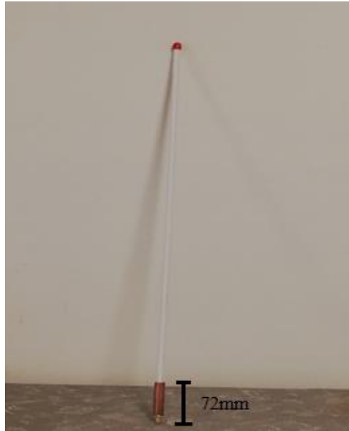
Figure 4.14: DIY collinear antenna with 72 mm longer diepole.
