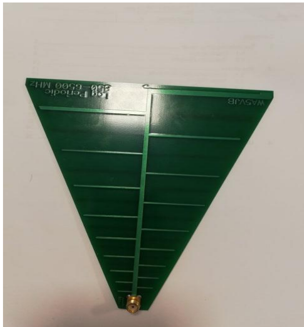
Figure 4.12: ANT3 (WA5VJB Log-Periodic antenna). Its frequency range is 850 - 6500 MHz, i.e. including ADS-B at 1090 MHz.
