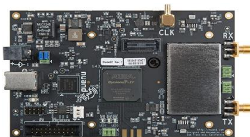
Figure 3.1: Photograph of Nuand bladeRF x115 SDR board. The board builds around a Cyclone IV FPGA (in the middle), LMS6002D radio front-end (right, under the metallic shield), and Cypress FX3 USB 3.0 interface (left) [34].
