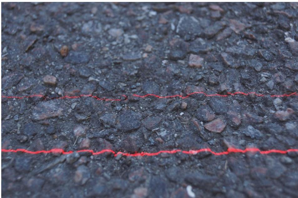
*Figure 2.1 Image captured by the scanner camera with multiple lasers [66 (III)].*
