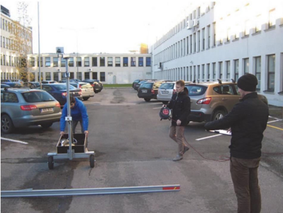
*Figure 3.20 Comparative measurements of real road transverse profile.*
