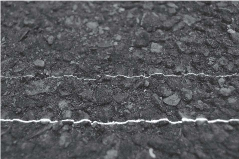
*Figure 2.2 Red channel image from the laser scanner camera [66 (III)].*
