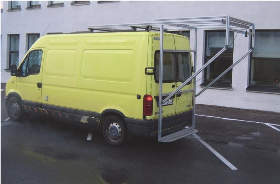
*Figure 5.4 Measurement system with camera and laser installed on van.*
