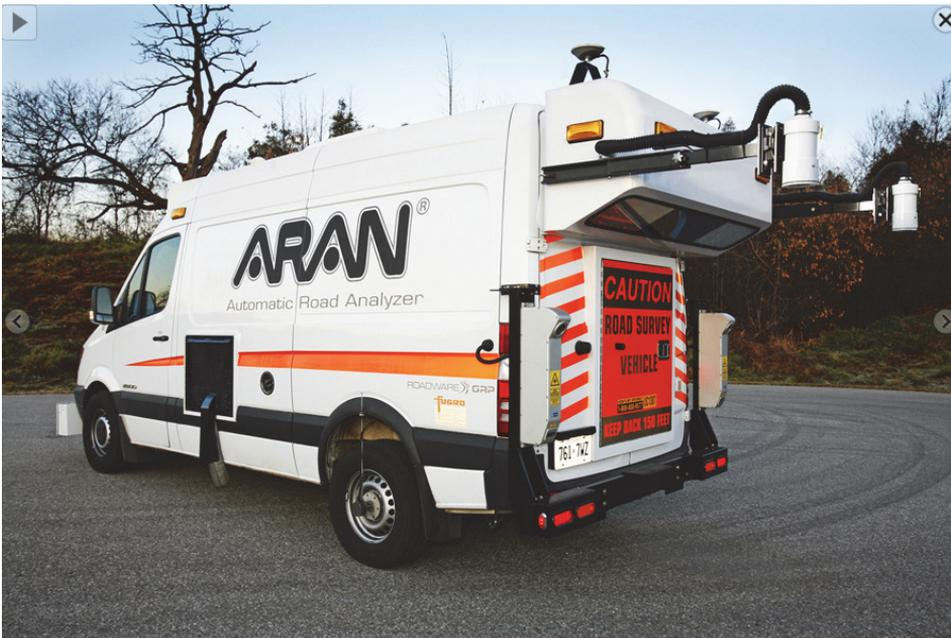
Figure 0.1 Example of „Furgo Roadware” road measurement system [1].
