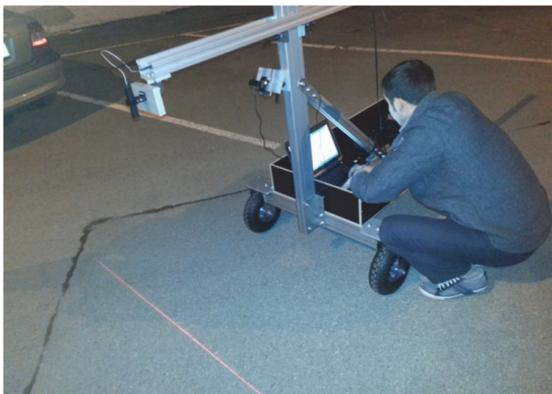
Fig. 4 Mobile test platform with adjustable camera and laser.
