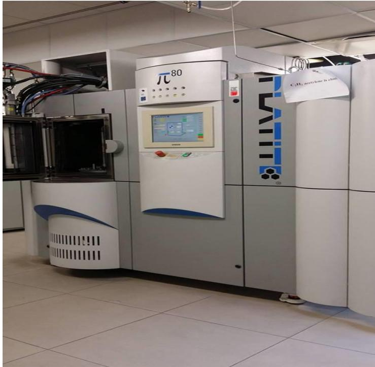
Figure 3.1: The Platit  $\pi$ 80 deposition system.
