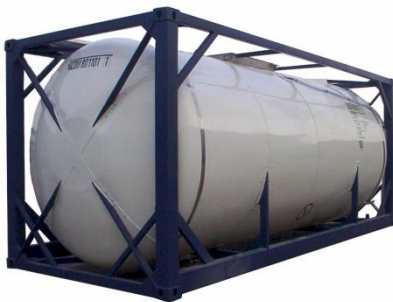
Figure 3. Typical tank container („Asia Tank Container Association“ homepage, 2015)
