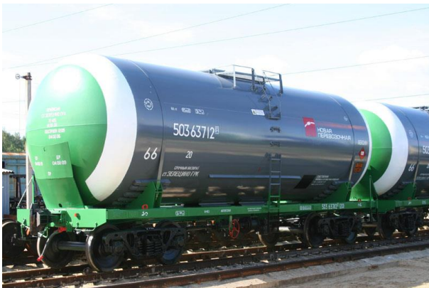
Figure 1. Typical rail tank car (“Globaltrans” homepage, 2015)
