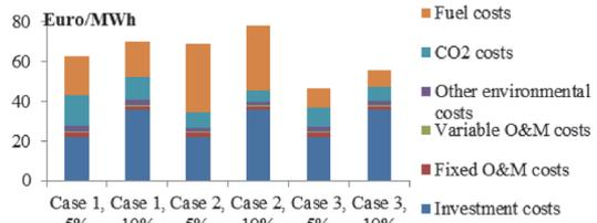
Figure 7. Levelized cost of generating electricity
