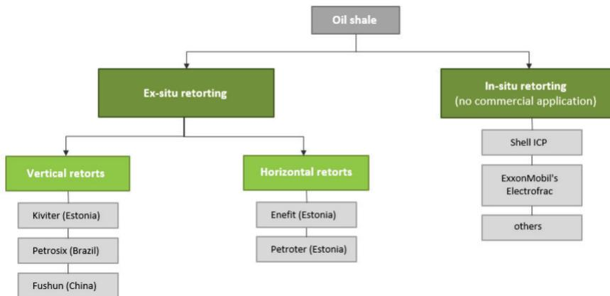
Figure 5. Oil shale retorting technologies [2].
