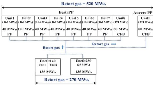
Figure 1. Thermal capacities of the Eesti and the Auvere power plants available for the utilization of the retort gas
