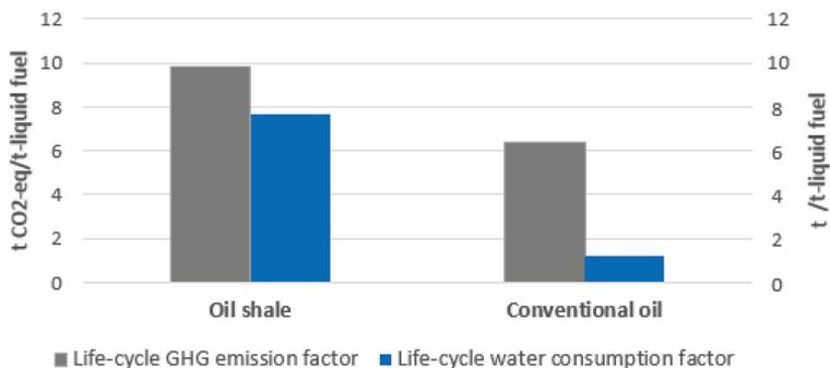
Figure 6. The life-cycle GHG emissions and water consumption of the production of liquid fuels from oil shale and conventional oil [22].
