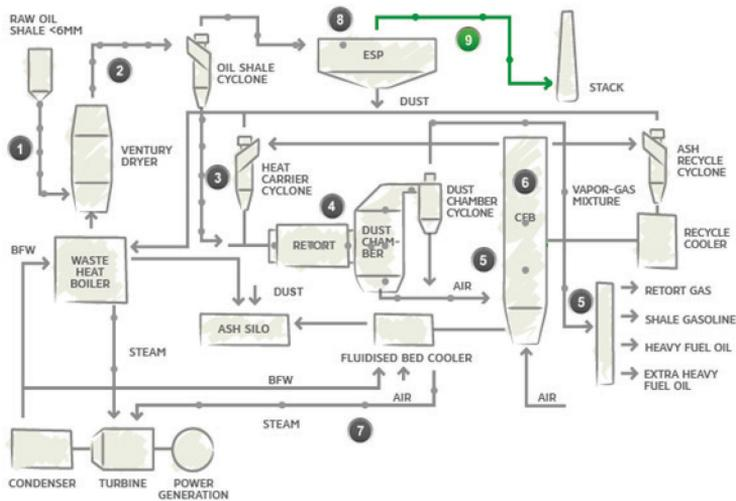
Figure 8. Process diagram of the Enefit280 oil shale retorting technology [26].
