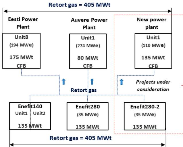
Figure 9. Expected thermal capacities to produce and utilize retort gas in Eesti Energia’s energy complex after 2030.
