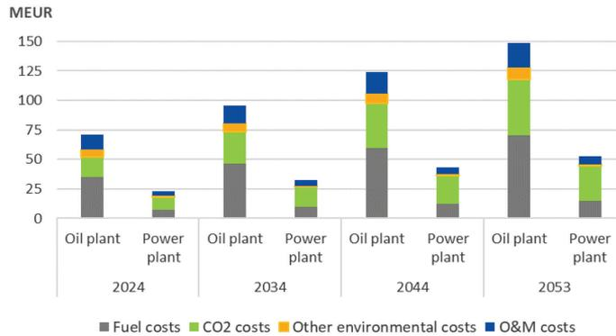
Figure 15. Operating costs of potential projects of a shale oil production plant and an oil shale power plant.
