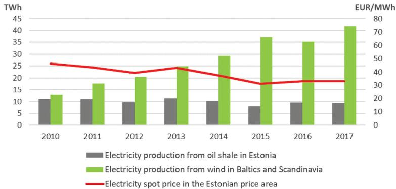
Figure 1. Electricity production from oil shale and wind in the Nordic and Baltic regions [12], [13].
