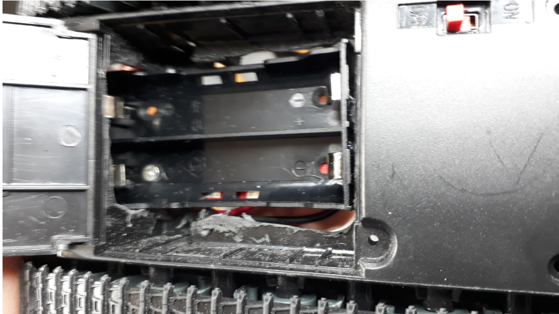
Figure 6. To fit the battery hold into the chassis, further modifications had to be made.
