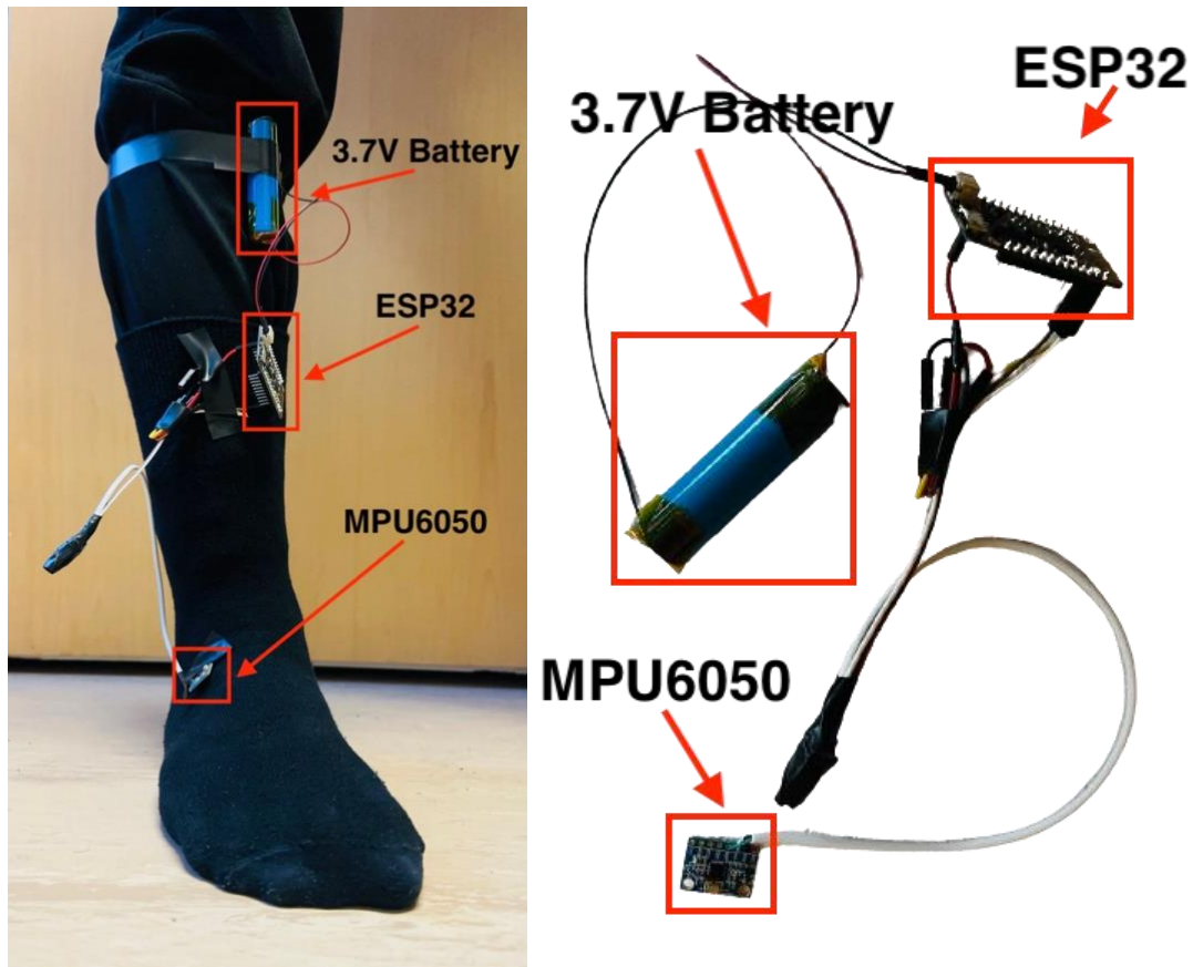
Figure 4. Placement of MPU6050 and ESP32 for Steppage Gait Analysis
