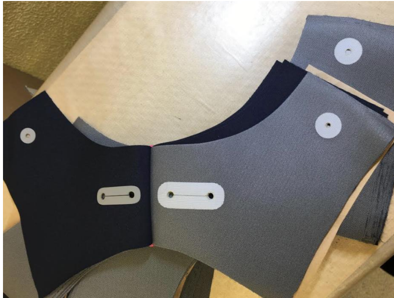
Figure 3.3 Examples of laser cut hood openings for cord and cord fixator (images provided by Ursuit Baltics AS)
