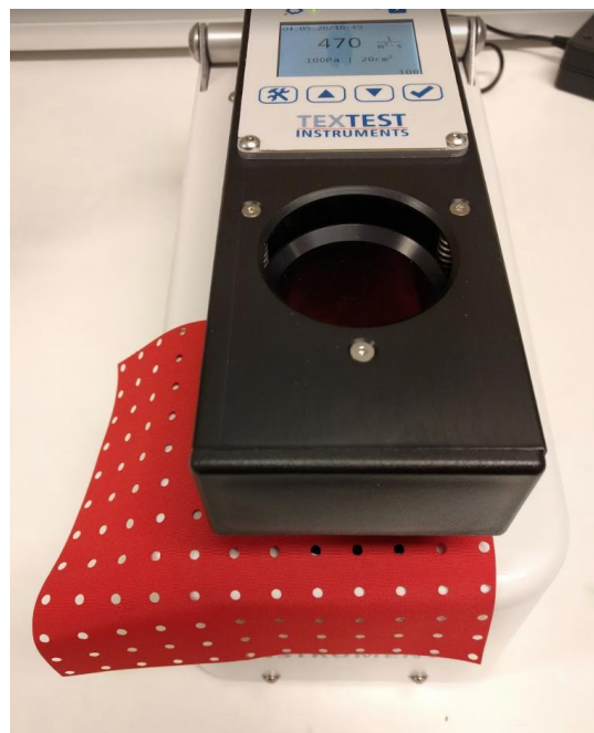
Figure 5.5 Measuring air permeability of the laser cut samples. 10 random locations were chosen for registering the result
