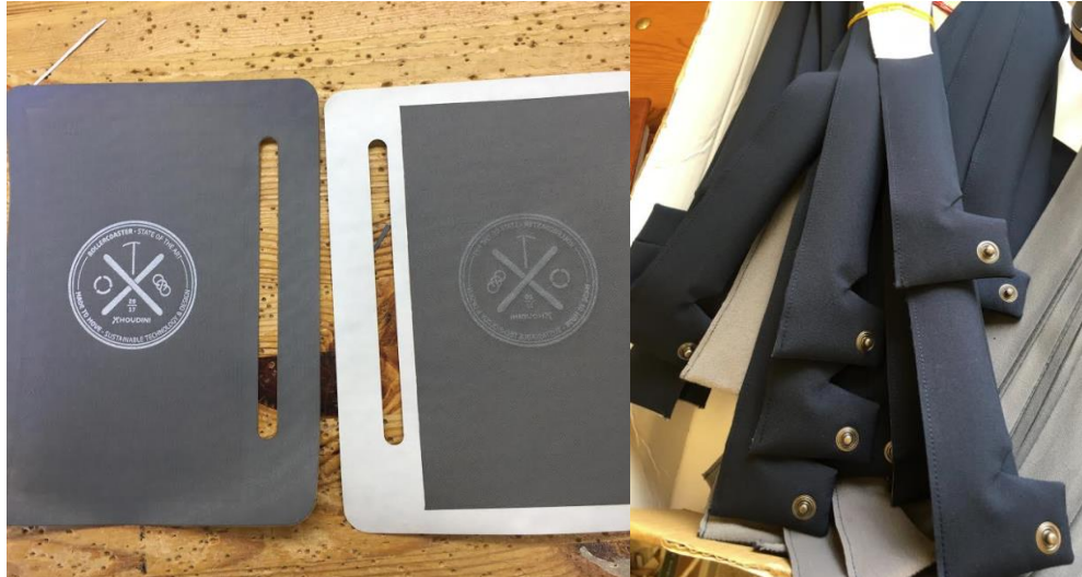
Figure 3.1 Examples of laser cut details: pocket piece (left) and front plackets (right) that have laser cut reinforcing lining pieces (images provided by Ursuit Baltics AS)
