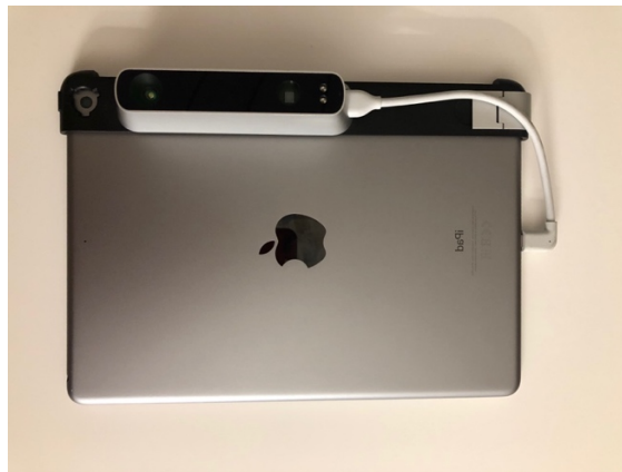
Figure 7. Structure Sensor scanner attached to the iPad. Source: the author.
