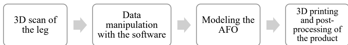
Figure 5. Additive manufacturing of AFO. Source: the author.
