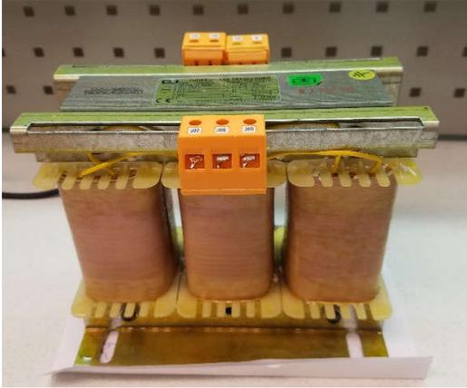
Figure 2.1 The real model of 3 phase power transformer (0,5 KVA; 380 V/110 V)
