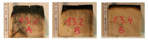
Figure 6-6. The cut cross-section of timber specimens protected by 10-, 20- and 40-mm plaster in TP1.
