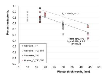
Figure 6-36. The protection factors for clay plaster systems (with reed mat) in relation to the thickness of plaster; obtained from the furnace tests.
