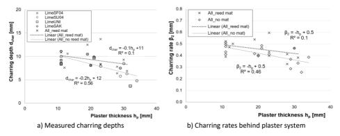
Figure 6-14. The charring depths and rates behind plaster systems obtained from cone heater tests (50 mm timber elements) in TP3.
