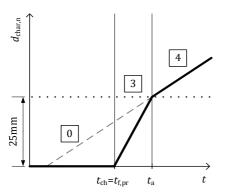
c) Initially protected sides of timber members when  $t_{f,pr} = t_{ch}$
