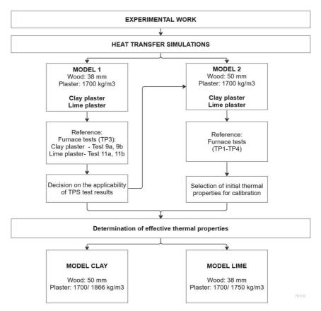
Figure 7-1. The concept map about the heat transfer simulations.
