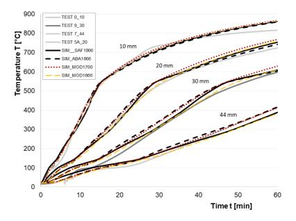
Figure 7-19. Comparison of temperature curves obtained from furnace tests and simulations with calibrated and modified thermal properties for clay plaster systems.
