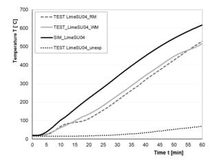
Figure 7-5. Comparison of temperature measurements between furnace tests (Test 11a, Test 11b) and simulations based on the TPS test results – 30 mm thick lime plaster systems.
