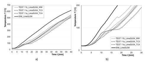
Figure 7-6. Comparison of temperature curves between furnace tests (Test 11a, Test 11b) and simulations based on the TPS test results – 30 mm thick lime plaster systems: a) Temperature curves up to 60 minutes; b) Close-up of the curves around 100°C.
