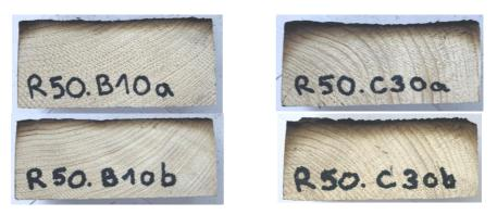
Figure 6-16. Residual cross-sections of timber specimens (50 mm) from double-testing after cone heater tests when protected by plaster: Left – 10 mm lime plaster; Right – 30 mm lime plaster.
