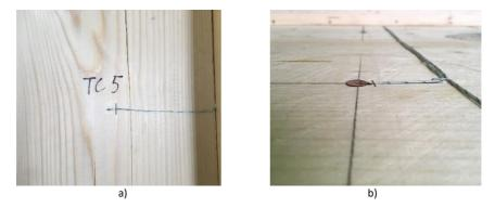
Figure 5-16. Close-up on the fixation of thermocouples (TC) on the exposed side of the timber elements before the application of plaster systems: a) TP1 and TP2; b) TP3 and TP4.
