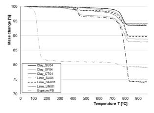
Figure 5-4. TGA test results of the relationship between mass loss and temperature.
