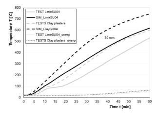
Figure 7-8. Comparison of mean temperature values between 30 mm thick clay and lime plaster systems (with a reed mat) obtained from furnace tests (TP3) and simulations.
