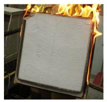
a) Test 10a – LimeSAK - Plaster surface after the removal of the test specimen from furnace.
