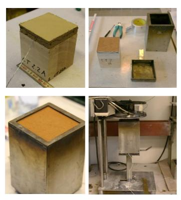
*Figure 5-11. The preparation and fixation of a test specimen in the cone heater tests.*
