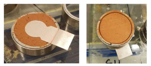
Figure 5-5. Preparation of test samples for TPS method: Left – MICA sensor fixed on one of the sample halves; Right – Test specimen after hardening and before the removal of the metal cylinder.
