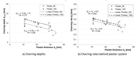
Figure 6-15. Comparison of the charring depths and rates behind plaster systems in relation to the depth of the timber elements (50 mm and 100 mm) in TP3.
