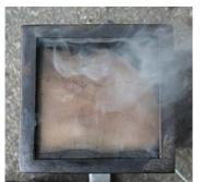
c) View of the plasters' surface after its removal from furnace and before extinguishment
