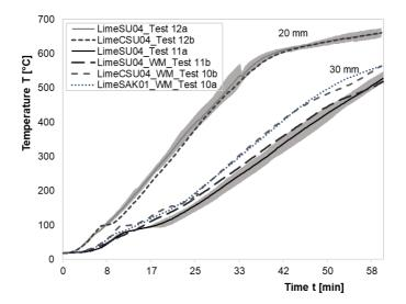
Figure 6-31. Mean temperature curves measured at the interface of plaster and timber in TP3.
