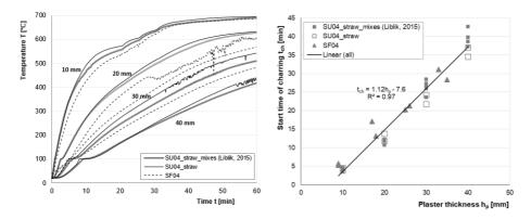
Figure 6-4. Mean temperature measurements and start time of charring obtained from cone heater tests in TP1.
