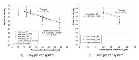
Figure 8-6. Furnace tests results on the relationship between the plaster thicknesses and the determined protection factors: a) Clay plaster system; b) Lime plaster system.
