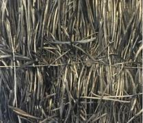
b) Close-up of the carbonised reed board after test.
