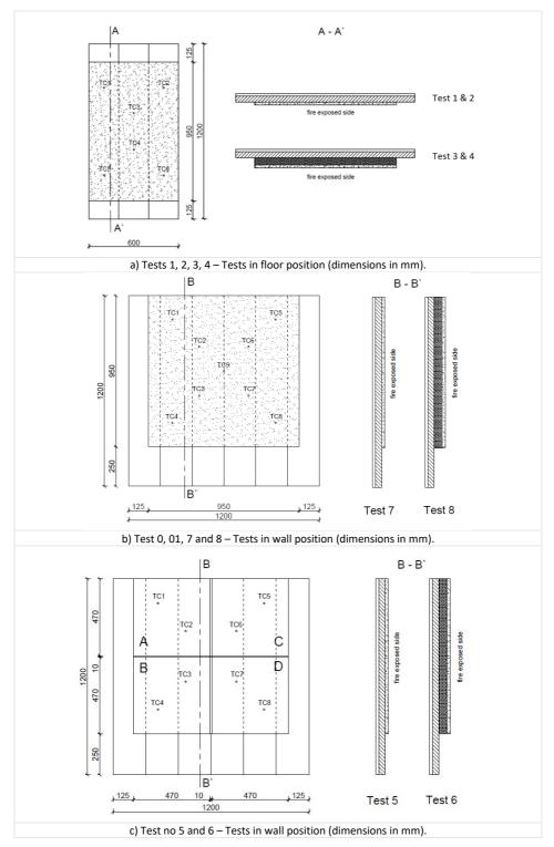
Figure 5-13. TP1 and TP2 – The layout of the fire-exposed side of the test specimens (with TC placements).
