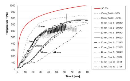
Figure 6-25. Mean temperature rise measured at the interface of clay plaster system and timber element in furnace tests.
