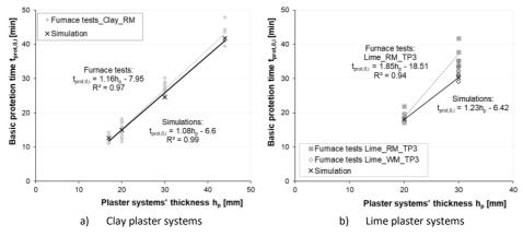
Figure 8-2. Comparison of the basic protection times determined by simulations and tests.
