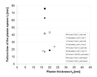
Figure 6-39. The fall-off times of clay plaster systems obtained from furnace tests, accompanied by estimations based on calculations.
