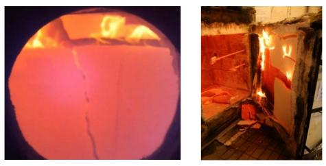
Figure 6-20. Documentation of Test 7 (44mm thick clay plaster system) during testing, approx. a minute before termination of the test (Left) and after its removal from furnace (Right).
