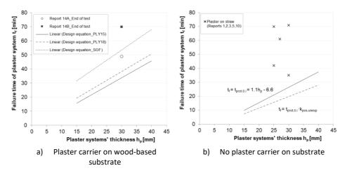
Figure 8-8. Comparison of failure times of clay plaster obtained from test reports and calculations.
