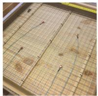
d) Wire mesh on timber panel in TP3
