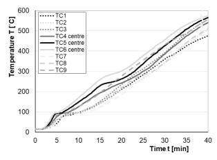
Figure 6-32. Temperature measurements at the interface of lime plaster system and timber element in Test 15 (TP4).
