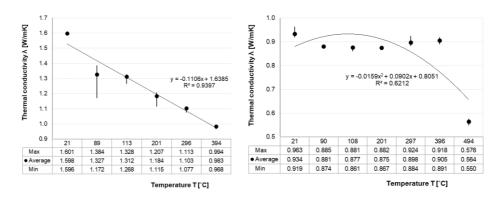
Figure 5-7. Thermal conductivity of clay plasters as determined by TPS tests: Left – ClaySU04; Right – ClaySF04.
