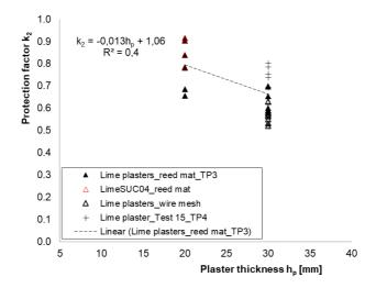
Figure 6-42. The protection factors for lime plaster systems obtained from the furnace test results.
