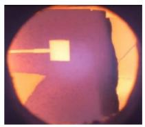
b) Detachment of first plaster coats after 43 minutes of fire exposure.
