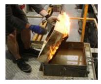
Figure 5-21. Cooling down the test specimens after its removal from furnace: Left – Furnace test in TP2; Right – Test specimen in TP3.
