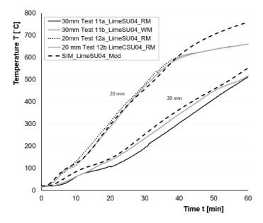
Figure 7-22. Comparison of temperature curves obtained from the furnace tests (TP3) for LimeSU04 plaster systems and simulations with (modified) effective thermal properties.
