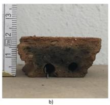
Figure 6-24. Documentation of the test specimen of Test 13 in TP4 during and after the fire test: a) View of the ceiling through furnace window, 3 minutes before the fall-off of the plaster system. b) A piece of the plaster system after fire test.
