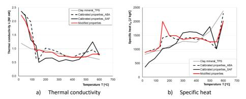
Figure 7-18. Comparison of the thermal properties determined by TPS tests (Küppers et al., 2018), calibrations and modifications for clay plaster systems.
