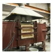
Figure 5-20. Preparation of test specimens for furnace testing: Left – Sides of plaster fixed with aluminum tape; Right – Test specimen fixed in furnace in TP3.
