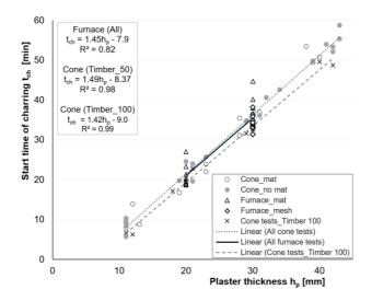
Figure 6-49. Comparison of start times of charring of timber protected by lime-based plaster system obtained from cone and furnace tests of TP3.
