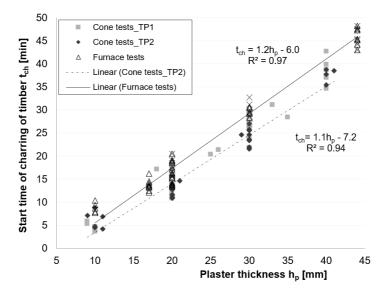
Figure 6-46. Comparison of start times of charring of timber protected by clay plaster system and reed mat as a plaster carrier.
