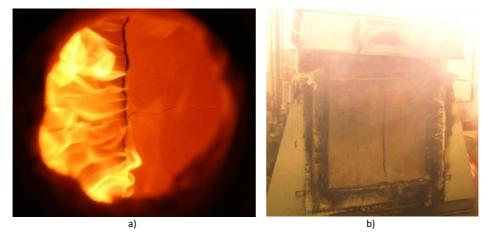
Figure 6-21. Documentation of Test 0 in TP1 during and after the termination of the fire test: a) View of the plaster systems' surface through the furnace window at 65 minutes of fire testing. b) Plaster attached to the furnace walls after the removal of the test specimen from furnace.
