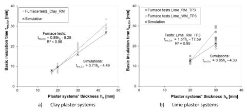
Figure 8-4. Comparison of test results and insulation times determined by simulations.
