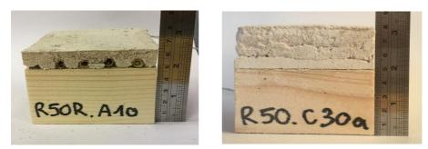
Figure 6-11. Test specimens prepared for the cone heater tests in TP3: Left – 10 mm thick lime plaster with a reed mat on timber specimen; Right – 30 mm thick lime plaster without reed mat.
