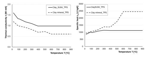
Figure 7-10. Comparison of the thermal properties obtained from TPS tests for 'ClaySU04' and 'Clay mineral' used as input for Model 2: Left – Thermal conductivity; Right – Specific heat.
