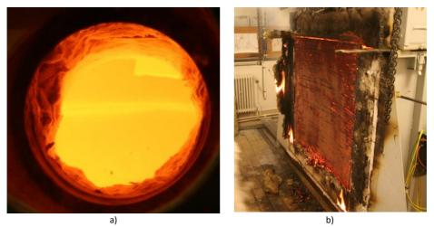
Figure 6-22. Documentation of Test 01 during and after the termination of fire test: a) View of the surface of plaster at 86 minutes of fire testing through the furnace window. b) Plaster attached to the furnace walls after the removal of the test specimen from furnace.
