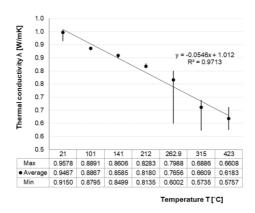
Figure 5-8. Thermal conductivity of lime plaster (LimeSU04) as determined by TPS tests.
