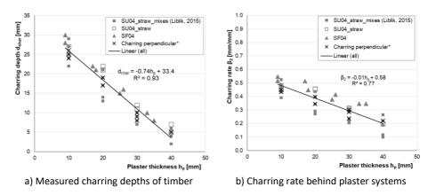
Figure 6-5. The charring performance of timber in relation to the plasters' thickness in TP1.
