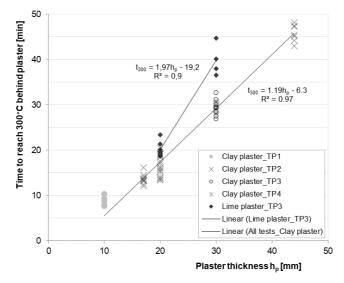
Figure 6-44. Comparison of furnace test results to reach the start time of charring behind clay and lime plaster systems.
