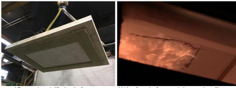
a) Test specimen is lifted to the furnace.
