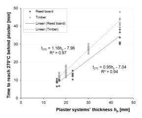
Figure 8-5. Comparison of test data to reach 270°C behind the plaster systems on timber element and reed board.
