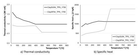
Figure 7-2. Comparison of mean values of thermal properties obtained from TPS tests and used for simulations in Model 1 – Clay plasters.
