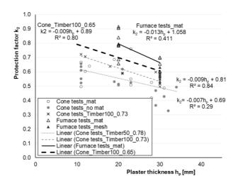
Figure 6-50. Comparison of protection factors of lime-based plaster systems obtained from cone and furnace tests of TP3.
