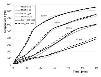
Figure 7-16. Comparison of temperature curves obtained in furnace and simulations with calibrated thermal properties based on "Clay mineral" input (Küppers et al., 2018).
