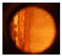
c) Test 11a – LimeSU04 - Visual cracks developed along the reed stems in a reed mat.
