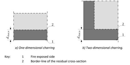
Figure 2-2. Notional charring depth d<sub>char,n</sub> (prEN 1995-1-2:2022)
