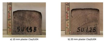
*Figure 6-9. The residual cross-sections of timber specimens documented after testing in TP2.*
