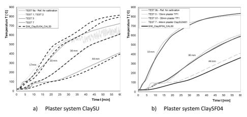
Figure 7-14. Comparison of temperature curves for different plaster thicknesses on timber determined by simulations using the effective thermal properties calibrated based on furnace tests in TP3 (Test 9a, Test 9b).
