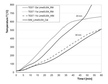
Figure 7-20. Comparison of furnace test results of lime plaster system LimeSU04 and first simulations based on calibrated thermal properties.
