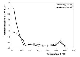
Table 7-5. Effective thermal properties based on the TPS test results (Clay mineral, constant density of 1866.65 kg/m<sup>3</sup>) and furnace test results from Test 5A.
