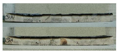
Figure 6-43. The cross-section of timber panels protected by 30 mm thick plasters: Above – LimeSU04 and reed mat; Below – LimeSU04 and wire mesh.
