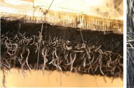
a) Reed board after its removal from furnace in a ceiling position.
