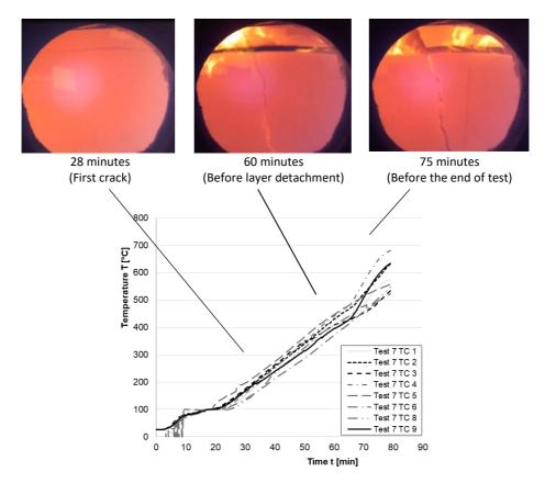
Figure A2-1. Temperature measurements at the interface of clay plaster (44 mm) and timber.
