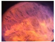
b) Test 4 – Reed board exposed to fire after the fall-off of plaster system.
