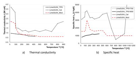
Figure 7-21. Comparison of thermal properties determined for lime plaster (LimeSU04).
