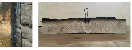
a) Clay plaster after the detachment of the outer plaster layers on timber.
