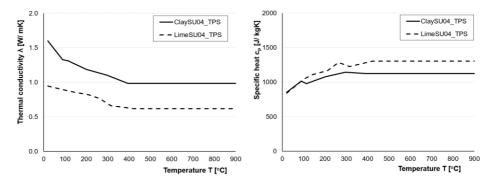
Figure 7-7. Comparison of the thermal properties of clay and lime plaster used as input for Model 1: Left – Thermal conductivity; Right – Specific heat.
