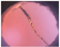
a) Test 3 – Fall-off of plaster system after 17 minutes of testing.
