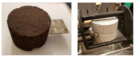
Figure 5-6. Documentation of test specimens after TPS tests: Left – Close-up of ClaySU04 after testing; Right – Cracking of LimeSU04 when tested in the electric furnace.
