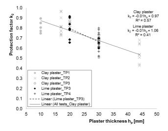
Figure 6-45. Comparison of protection factors between clay and lime-based plaster systems obtained from the furnace tests.
