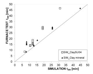
Figure 7-11. Relationship between the mean results of furnace tests and the first simulations on the time to reach 300°C on timber ( $t_{300}$ ) for clay plaster systems.
