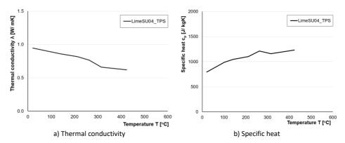
Figure 7-4. Mean temperature-dependent thermal properties obtained from TPS tests for lime plaster – LimeSU04.
