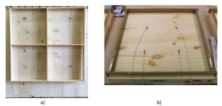
Figure 5-17. Temporary wooden frames fixed on timber element for the application of plaster: a) Framework fixed on timber element in TP2 (Test 6); b) Framework fixed on wooden panel in TP3.
