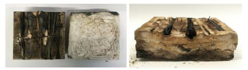
Figure 6-13. A test specimen after cone heater testing and cooled down with water: Left – Top view of the timber specimen from which the plaster system was removed and put aside; Right – A close up of the plaster system (incl. the reed mat), placed upside down.
