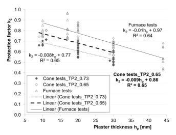
Figure 6-48. Comparison of protection factors of clay plaster systems.
