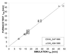
Figure 7-17. Comparison of the agreement between the times to reach the 300°C behind plaster system in furnace and simulations based on calibrated thermal properties (Table 7-5).
