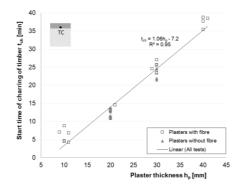
Figure 6-7. The start times of charring obtained from cone heater tests in TP2.
