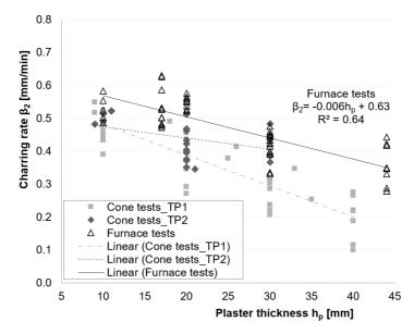
Figure 6-47. Comparison of charring rates of timber protected by clay plaster systems.
