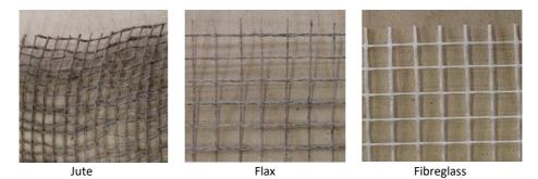
Figure 5-1. Types of reinforcement meshes used in plaster systems.
