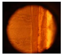
e) Test 12a – LimeSU04 on reed mat - Cracks developed after 17 minutes of testing.
