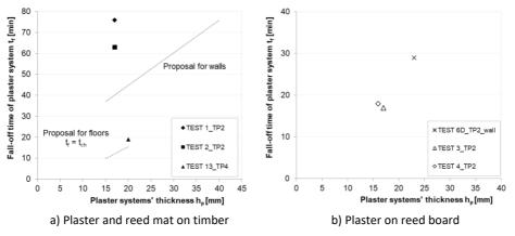
Figure 8-7. The failure times of clay plaster systems.
