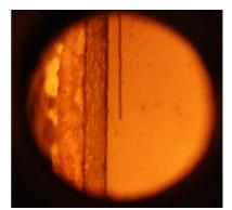
f) Test 12b – LimeCSU04 on reed mat - No visible cracks developed during the test.
