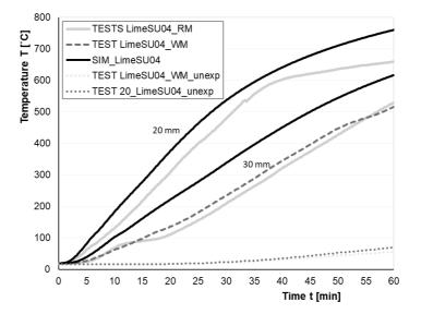
Figure 7-12. Comparison of temperature measurements obtained in furnace behind the lime plaster systems (with reed mat) and derived from the simulations of Model 2.
