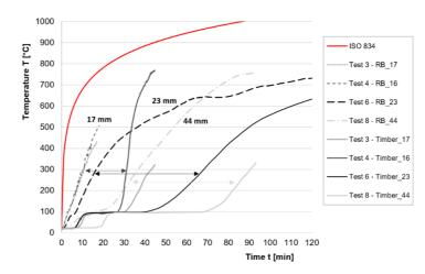
Figure 6-29. Mean temperature curves recorded on the fire-exposed side of the reed board (RB) and on the timber element (Timber) for each furnace test (Test 3, 4, 6, 8), protected by various clay plaster system thicknesses.
