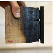
b) Plaster intact with timber after fire test
