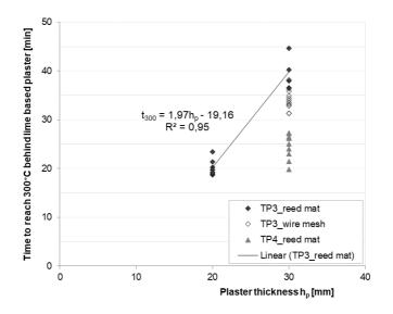
Figure 6-41. Relationship between the lime plaster systems' thickness and time to reach 300°C behind lime-based plasters tested in TP3 and TP4.
