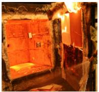
b) Test specimen after removal from the furnace.
