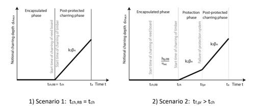
Figure 10-1. Charring models for plaster systems and reed board on timber structures.
