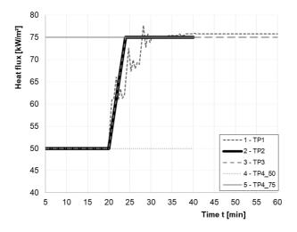
Figure 5-9. Heat flux scenarios used in cone heater tests.
