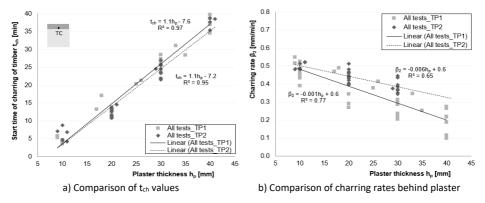
Figure 6-10. Comparison of test results obtained from TP1 and TP2.
