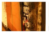
a) Plaster intact to timber after fire test
