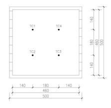
b) Test no 9, 10, 11,12 (dimensions in mm)
