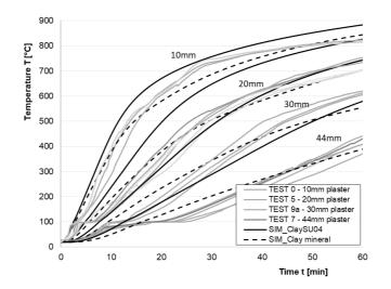
Figure 7-9. Comparison of temperature measurements obtained in furnace behind the clay plaster system (wall tests) and simulation results of Model 2.
