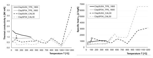
Figure 7-13. Comparison of thermal properties obtained from TPS tests and effective thermal properties determined by first calibrations.
