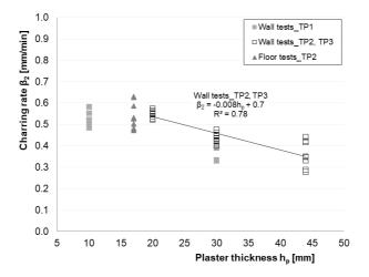
Figure 6-35. The charring rates of timber protected by clay plaster systems in relation to the thickness of plaster, determined in furnace tests.
