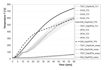
Figure 7-3. Comparison of temperature measurements recorded in furnace (Test 9a, Test 9b, TP3) and simulations based on TPS test results – clay plaster systems.
