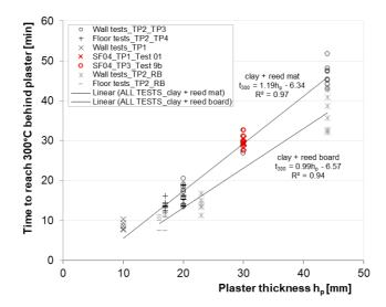
Figure 6-34. Relationship between the thickness of clay plaster systems and the time to reach 300°C behind plaster system in case of reed mat and on a reed board (\_RB).
