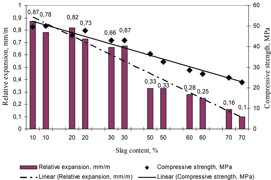
Figure 5.4.1 Sulfate resistance of Portland slag cements and slag cements ( $Al_2O_3$  content in slag  $S_1 = 17.95\%$ ,  $S_2 = 15.70\%$ )
