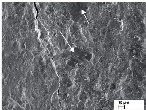
Figure 5.3.11 CEM II/A -  $T_K$  (20 %  $T_K$ ) paste cured for 91 days in the 4.4 %  $\text{Na}_2\text{SO}_4$  solution. Ettringite nests.
