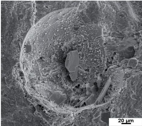
Figure 5.5.8 CEM II/B-M (20% $T_T$ + 5%S + 10%L) mortar stored for 91 days in the 4.4 %  $Na_2SO_4$  solution. Near the surface large air voids are visible. Ettringite crystals are growing.
