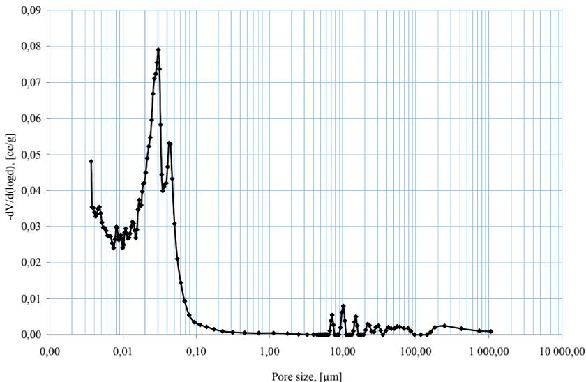
Figure 5.1.7 Pore size distribution of CEM I paste after exposure to the 4.4 %  $\text{Na}_2\text{SO}_4$  solution for 91 days
