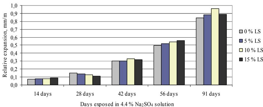
Figure 5.2.1 Relative expansion values of Portland limestone cements with limestone content 5, 10 and 15 % compared to Portland cement CEM I
