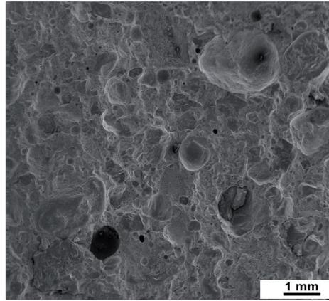
Figure 5.2.3 CEM II/A-L (10% L) mortar cured for 91 days in the saturated  $\text{Ca}(\text{OH})_2$  solution. Many air voids with different sizes can be seen.
