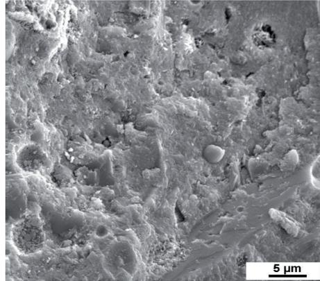
Figure 5.5.7 CEM II/B-M (20% $T_T$  + 5%S+10%L) mortar for 91 days in the saturated  $Ca(OH)_2$  solution. Cement stone is coarse in spots. In every void the secondary products are growing.
