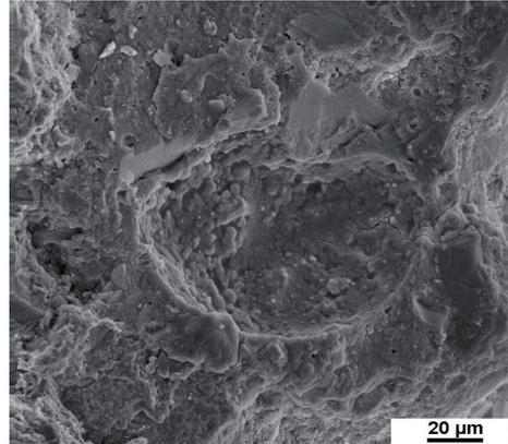
Figure 5.5.3 CEM V/B (50 % S + 20 % T<sub>T</sub>) mortar stored for 91 days in the 4.4 % Na<sub>2</sub>SO<sub>4</sub> solution. An air void. The cement stone is very dense.
