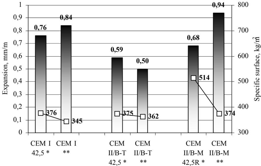
Figure 5.6.2 Comparative values of relative expansion of the Wittekindt test with commercial and laboratory made cements. \* - commercial cement, \*\* - laboratory cement
