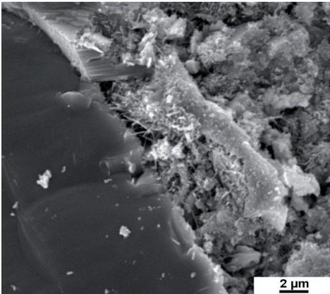
Figure 5.1.2 CEM I mortar cured for 14 days in the saturated Ca(OH)<sub>2</sub> solution. Crystals are growing into paste-aggregate interfacial zone.
