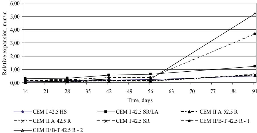
Figure 5.7.4 Relative expansion of commercial cement mortar specimens (10 x 40 x 160) mm in 1.1 %  $(NH_4)_2SO_4$  solution
