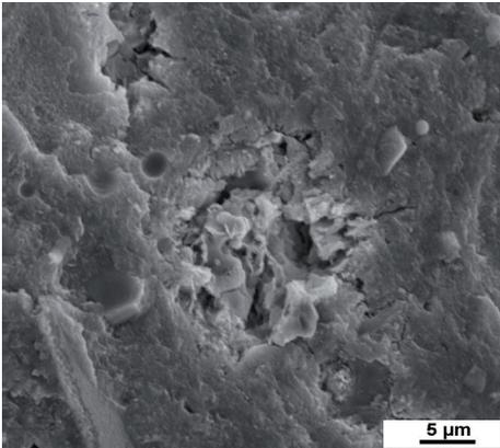
Figure 5.5.4 CEM V/B (50 % S + 20 % T<sub>T</sub>) mortar stored for 91 days in the 4.4 % Na<sub>2</sub>SO<sub>4</sub> solution. Air void filled with secondary reaction products.
