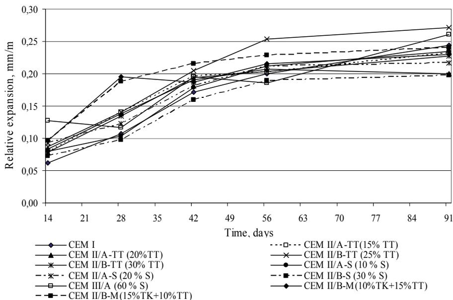
Figure 5.7.1 Relative expansion of cement mortar specimens (10 x 40 x 160) mm in 1 %  $MgSO_4$  solution
