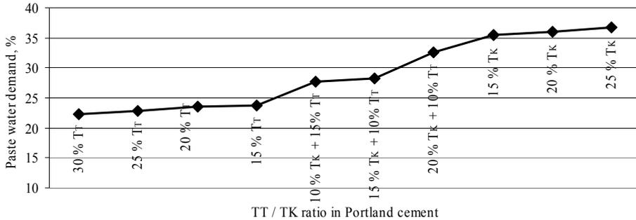
Figure 4.1.4 Increase of paste water demand in cement depending on  $T_T$  and  $T_K$  proportion
