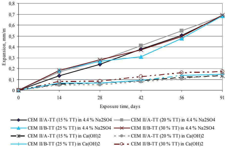
Figure 5.3.1 Expansion of Portland burnt shale cements depending on T<sub>T</sub> content in cement in the 4.4 % Na<sub>2</sub>SO<sub>4</sub> and in the saturated Ca(OH)<sub>2</sub> solutions
