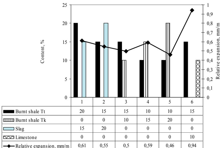
Figure 5.5.1 Relative expansion of multicomponent Portland composite cements depending on cement composition
