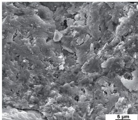
Figure 5.1.5 CEM I mortar 91 days in the 4.4 % Na<sub>2</sub>SO<sub>4</sub> solution. The cement stone is tight. Pores of cement stone are filled with gypsum and ettringite crystals.
