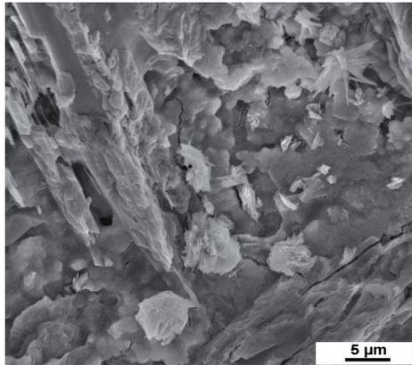
Figure 5.1.3 CEM I mortar stored for 91 days in the 4.4 % Na<sub>2</sub>SO<sub>4</sub> solution. Figure shows the bottom of an air void. The hydration products are cotton-shaped CSH gel, plated-shaped Ca(OH)<sub>2</sub>, gypsum and ettringite. Cracks in the bottom.
