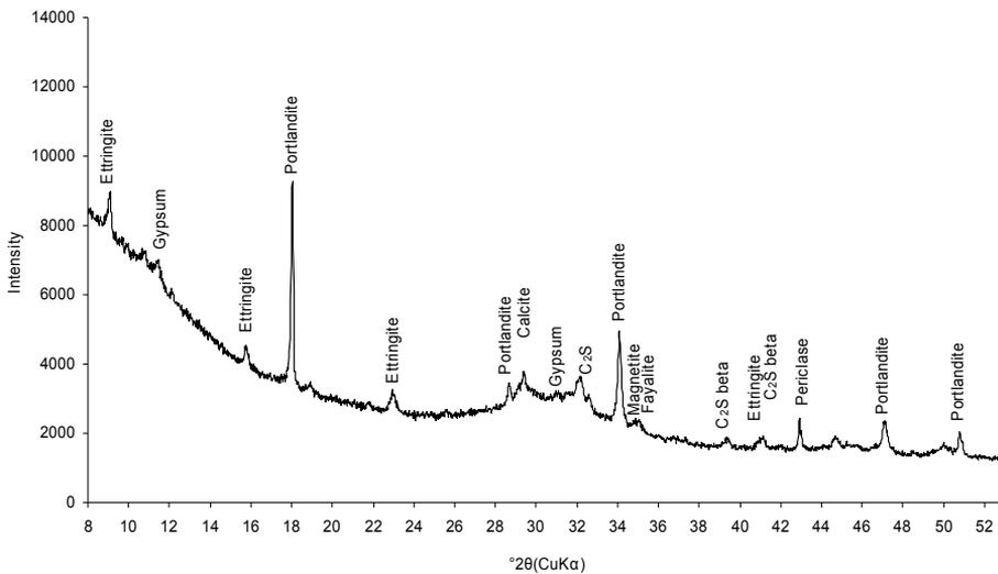
Figure 5.4.7 XRD analysis of slag cement CEM III/A (60 % S) paste after exposure to the 4.4 %  $\text{Na}_2\text{SO}_4$  solution for 91 days
