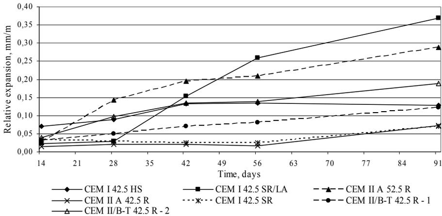
Figure 5.7.2 Relative expansion of commercial cement mortar specimens (10 x 40 x 160) mm in 1 % MgSO<sub>4</sub> solution
