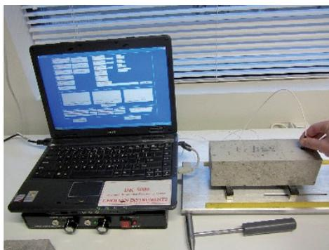
Figure 3.7.1 The device for measuring dynamic modulus of elasticity of mortar or concrete
