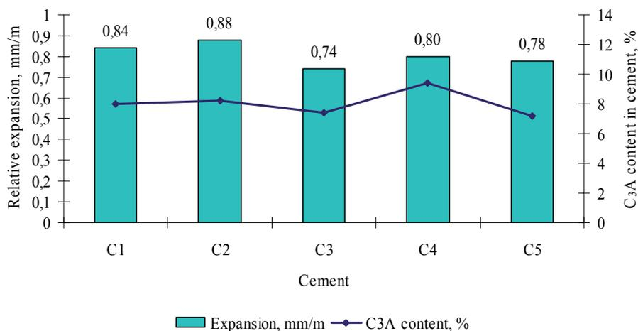
Figure 5.1.1 Relative expansion of Portland cements made with clinkers  $C_1...C_5$  depending on the  $C_3A$  content of cement ( $SO_3$  content of all cements is 3.5 %)
