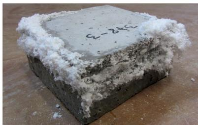
Figure 6.4.3 Concrete specimen made with CEM III/A (70 % S) cement. Absorption time 49 days in 4.4 %  $\text{Na}_2\text{SO}_4$
