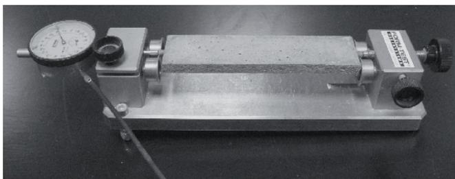
Figure 3.1.1 Test specimen and testing device for the determination of the sulfate resistance of the cement mortar by the Wittekindt method
