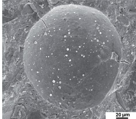
Figure 5.4.6 CEM III/A (60 % S) mortar stored for 91 days in the 4.4 %  $\text{Na}_2\text{SO}_4$  solution. Air voids are empty.
