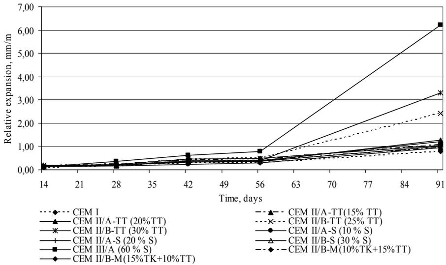
Figure 5.7.3 Relative expansion of cement mortar specimens (10 x 40 x 160) mm in 1.1 %  $(\text{NH}_4)_2\text{SO}_4$  solution
