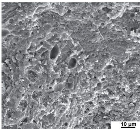
Figure 5.3.3 CEM II/A- $T_T$  (20%  $T_T$ ) mortar cured for 14 days in the saturated  $Ca(OH)_2$  solution. The particles of burnt shale  $T_T$  are visible.
