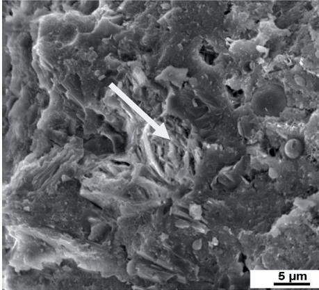
Figure 5.3.5 CEM II/A-T<sub>T</sub> (20% T<sub>T</sub>) mortar stored for 91 days in the 4.4 % Na<sub>2</sub>SO<sub>4</sub> solution. Air void filled with secondary reaction products.
