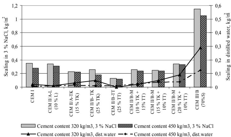
Figure 6.2.1 Scaling of concrete in 3 % NaCl and in distilled water after 56 cycles
