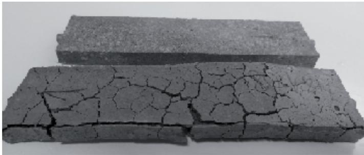
Figure 5.2.7 Examples of specimens after 91 days of exposure of CEM II/A-L (15 % L) in the 4.4 %  $\text{Na}_2\text{SO}_4$  solution and in the saturated  $\text{Ca}(\text{OH})_2$  solution
