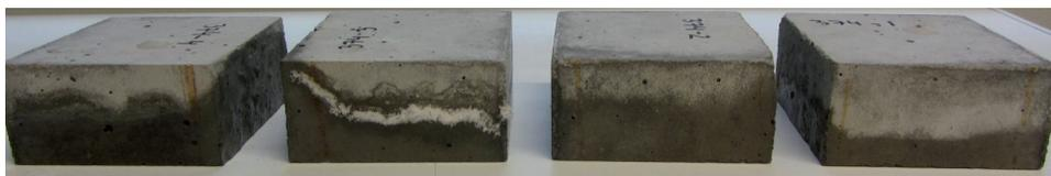
in 3.6%  $\text{MgSO}_4$  solution    in 4.4%  $\text{Na}_2\text{SO}_4$  solution    in 3%  $\text{NaCl}$  solution    in water
