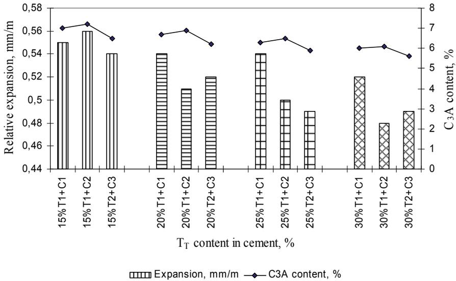
Figure 5.3.2 Relative expansion of Portland burnt shale T<sub>T</sub> cements depending on cement C<sub>3</sub>A and burnt shale T<sub>T</sub> content. Cements are made of various clinkers (C<sub>1</sub>, C<sub>2</sub> and C<sub>3</sub>) and burnt shales (T<sub>T</sub>1 and T<sub>T</sub>2)
