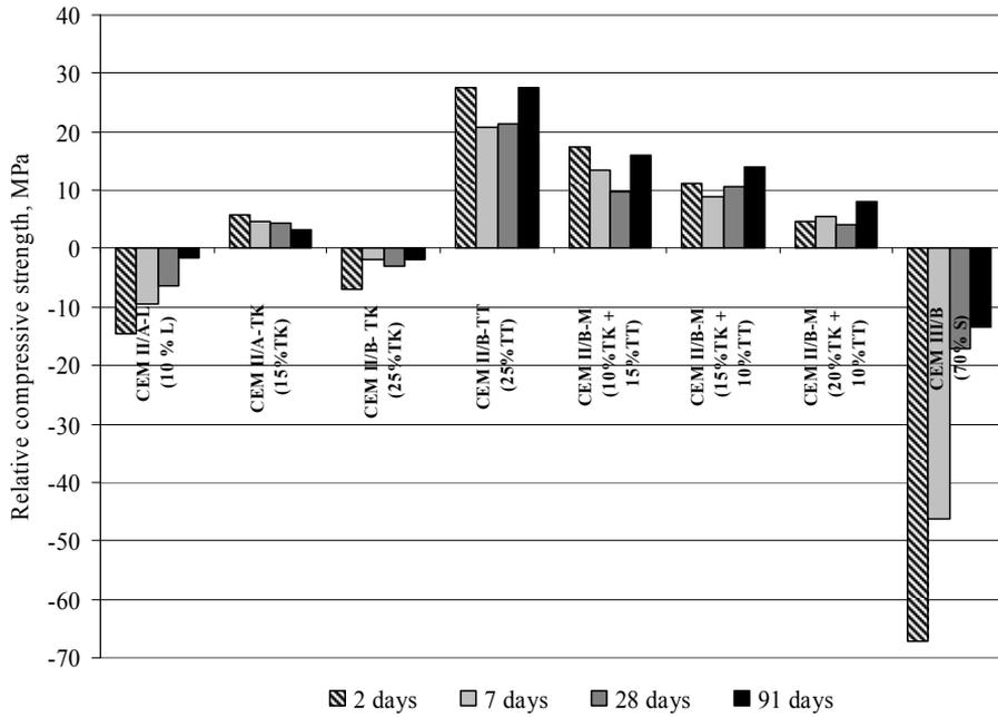
Figure 6.1.1 Relative compressive strength of concrete compared to CEM I (Cement content in concrete 320 kg/m³)
