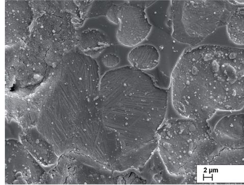
Figure 5.3.13 CEM II/A - T<sub>K</sub> (20 % T<sub>K</sub>) paste stored for 91 days in the 4.4 % Na<sub>2</sub>SO<sub>4</sub> solution. Near the surface of specimen gypsum was detected up to the depth of 385 μm.
