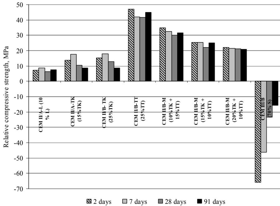
Figure 6.1.2 Relative compressive strength of concrete compared to CEM I (Cement content in concrete 450 kg/m³)
