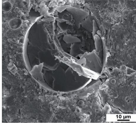
Figure 5.3.6 CEM II/A-T<sub>T</sub> (20% T<sub>T</sub>) mortar stored for 91 days in the 4.4 % Na<sub>2</sub>SO<sub>4</sub> solution. Air void filled with expanded products and void centered cracks.
