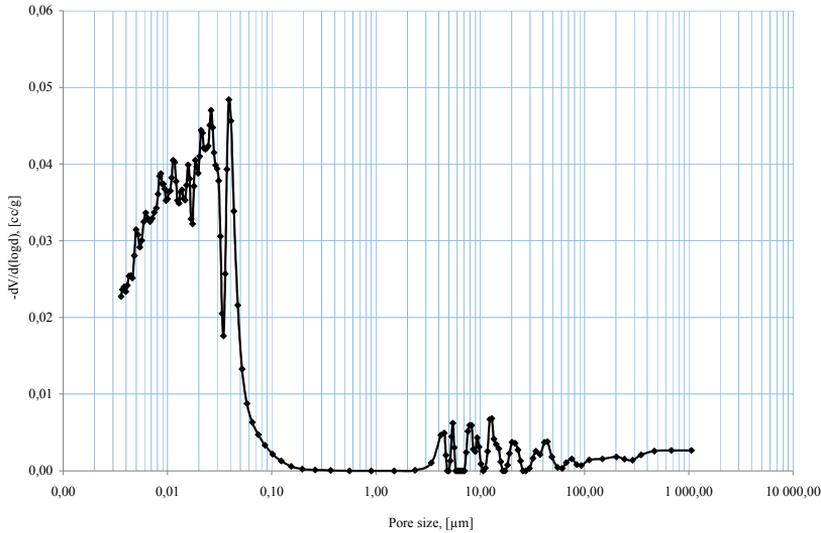
Figure 5.2.8 Pore size distribution of Portland limestone cement CEM II/A-L (10 % L) paste. Specimens were stored in the 4.4 %  $\text{Na}_2\text{SO}_4$  solution for 91 days
