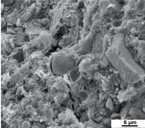
Figure 5.5.6 CEM II/B-M (20% $T_T$  + 5%S + 10%L) mortar cured for 14 days in the saturated  $Ca(OH)_2$  solution.
