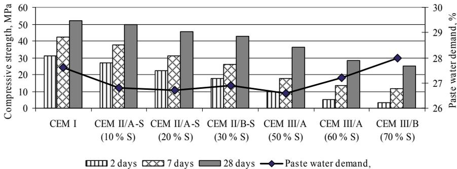
Figure 4.1.5 Compressive strength and paste water demand of Portland slag cements and slag cements compared to CEM I
