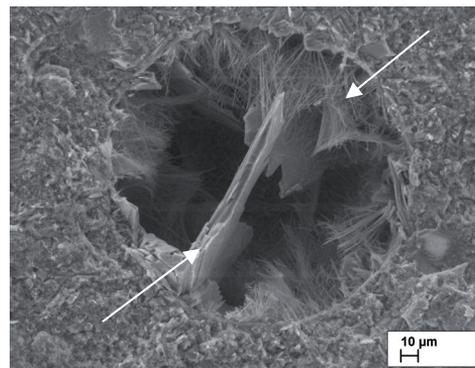
Figure 5.3.12 CEM II/A -  $T_K$  (20 %  $T_K$ ) paste stored for 91 days in the 4.4 %  $\text{Na}_2\text{SO}_4$  solution. An air void partly filled with ettringite needles. In the middle is  $\text{Ca}(\text{OH})_2$  crystal.
