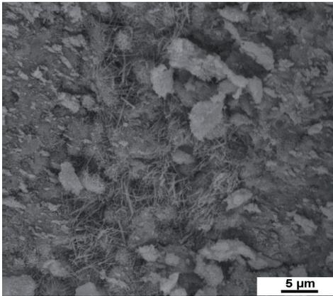
Figure 5.4.3 CEM III/A (60 % S) mortar cured for 14 days in the Ca(OH)<sub>2</sub> solution. A great amount of needle-shaped ettringite.
