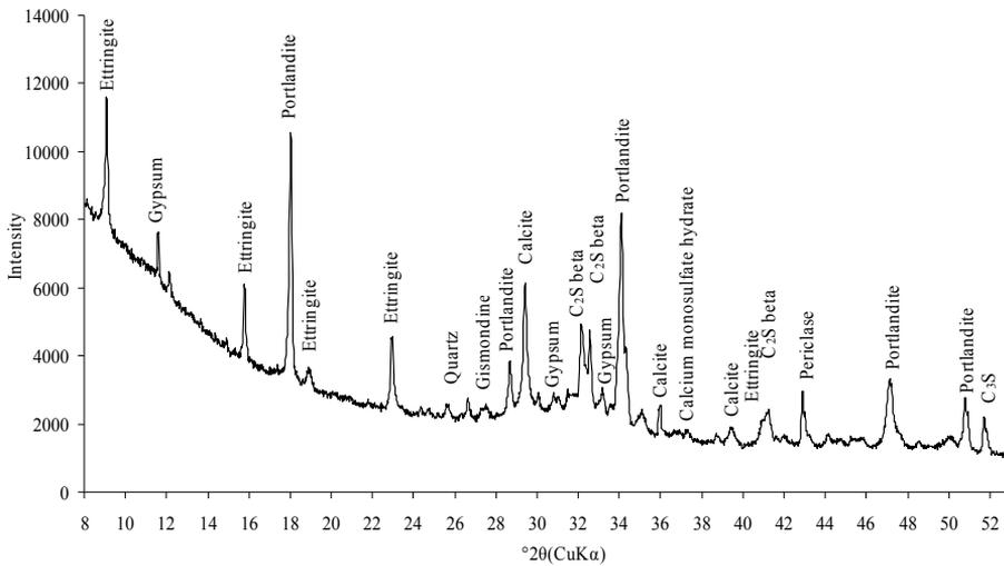
Figure 5.2.6 XRD analysis of Portland limestone cement CEM II/A-L (10% L) paste after exposure to the 4.4 %  $\text{Na}_2\text{SO}_4$  solution for 91 days
