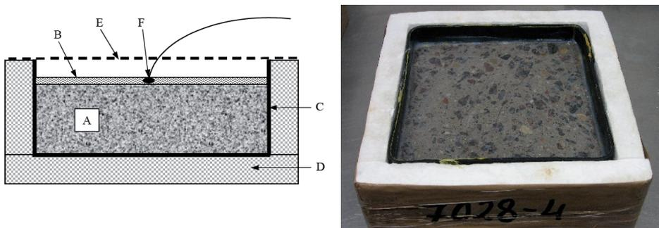
Figure 3.3.1 Concrete test specimen for determination freeze-thaw resistance. A - concrete specimen (150 x 150 x 50) mm, B - freezing medium (3 mm), C - rubber sheet for moisture insulation, D - polystyrene cellular plastic for thermal insulation, E - polyethylene sheet to prevent the freezing medium from evaporating F – temperature measuring device
