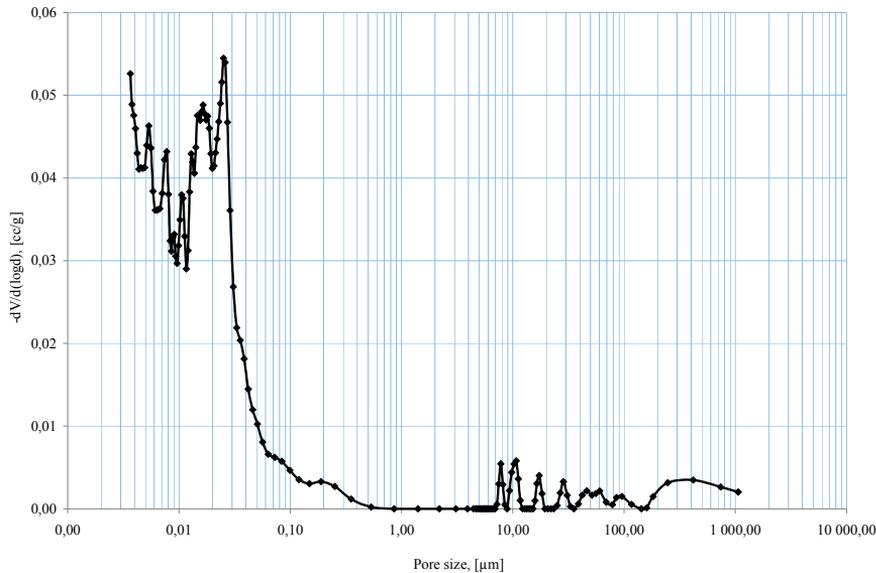
Figure 5.3.8 Pore size distribution of Portland burnt shale cement CEM II/A- $T_T$  (20 %  $T_T$ ) paste. Specimens were stored in the 4.4 %  $\text{Na}_2\text{SO}_4$  solution for 91 days
