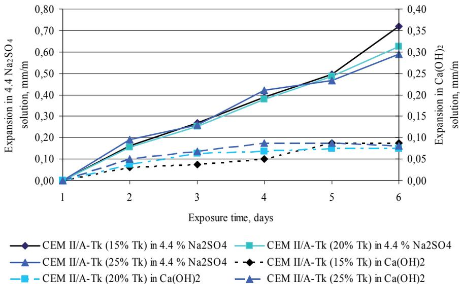
Figure 5.3.9 Expansion behavior of flat mortar prisms of Portland burnt shale  $T_K$  cements with 15%, 20% and 25%  $T_K$  immersed in the 4.4 %  $\text{Na}_2\text{SO}_4$  solution and in the saturated  $\text{Ca}(\text{OH})_2$  solution
