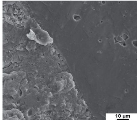
Figure 5.5.5 CEM V/B (50 % S + 20 % T<sub>T</sub>) mortar stored for 91 days in the 4.4 % Na<sub>2</sub>SO<sub>4</sub> solution. The paste-aggregate interfacial zone is tight.
