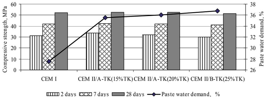
Figure 4.1.3 Compressive strength and paste water demand of Portland burnt shale  $T_K$  cements compared to CEM I
