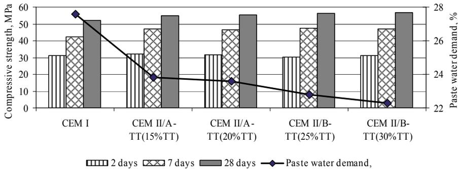
Figure 4.1.2 Compressive strength and paste water demand of Portland burnt shale  $T_T$  cements compared to CEM I
