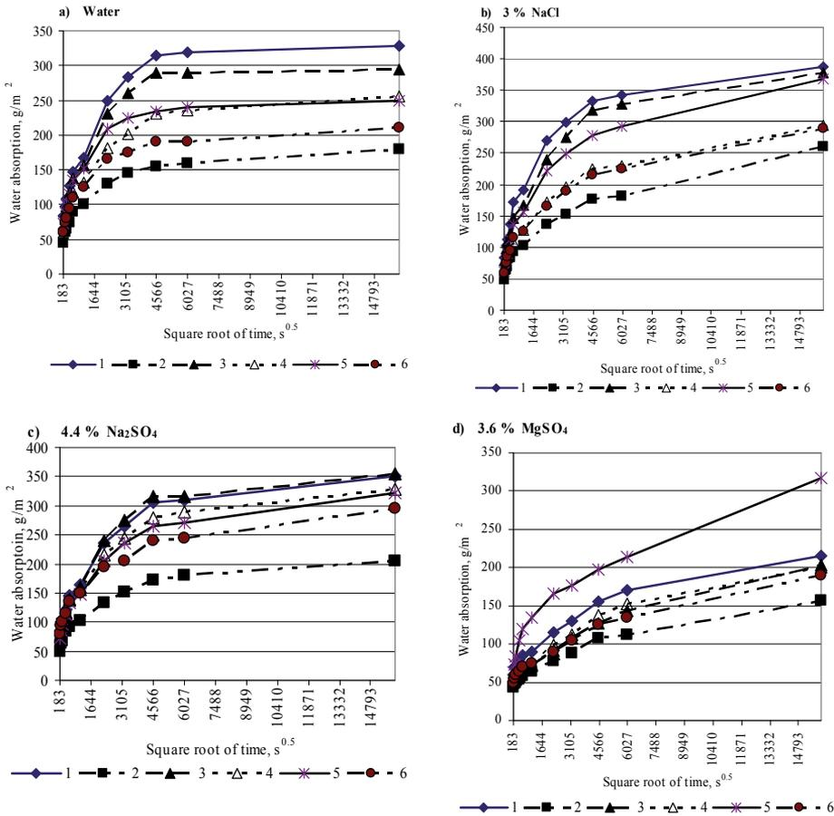
Figure 6.4.4. Water and salt absorption as a graph of  $(m_{s0,s} - m_{dry,s}) / A_s$  against the square root of the time immersed, in seconds for concretes made with several cements. a) in water, b) in 3 % NaCl solution, c) in 4.4 % Na<sub>2</sub>SO<sub>4</sub> solution, d) in 3.6 % MgSO<sub>4</sub> solution
