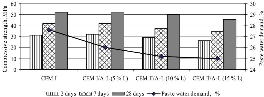
Figure 4.1.1 Compressive strength and paste water demand of Portland limestone cements compared to CEM I
