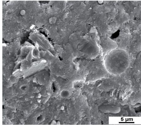
Figure 5.5.9 CEM II/B-M (20% $T_T$ + 5%S+10%L) mortar stored for 91 days in the 4.4 %  $Na_2SO_4$  solution. The structure is uneven.
