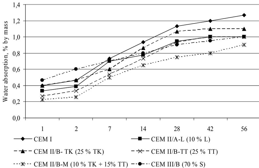
Figure 6.4.1 Water absorption of concretes
