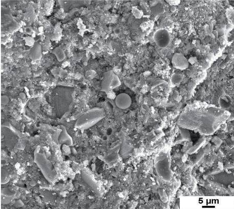
Figure 5.5.2 CEM V/B (50 % S + 20 % T<sub>T</sub>) mortar cured for 14 days in the Ca(OH)<sub>2</sub> solution. The spherical particles of slag and burnt shale T<sub>T</sub> are observable.
