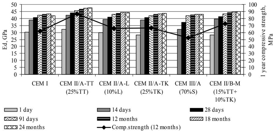
Figure 6.5.1 Dynamic modulus of elasticity up to two years and compressive strength after one year of storage in the 4.4 %  $\text{Na}_2\text{SO}_4$  solution of concrete specimens with dimensions 70 x 70 x 210 mm
