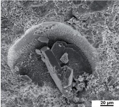
Figure 5.2.2 CEM II/A-L (10% L) mortar cured for 14 days in the saturated  $\text{Ca}(\text{OH})_2$  solution. Ettringite crystals grow at the surface of the mortar in voids.
