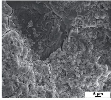
Figure 5.2.5 CEM II/A-L (10% L) mortar stored for 91 days in the 4.4 %  $\text{Na}_2\text{SO}_4$  solution. The structure is fragile with many cracks.
