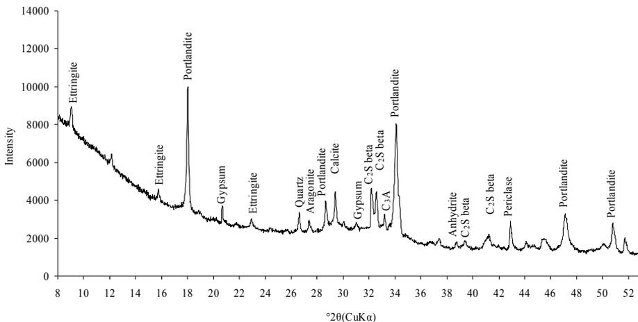
Figure 5.3.7 XRD analysis of Portland burnt shale cement CEM II/A-T<sub>T</sub> (20% T<sub>T</sub>) paste after exposure to the 4.4 % Na<sub>2</sub>SO<sub>4</sub> solution for 91 days
