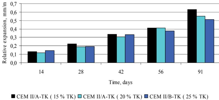
Figure 5.3.10 Sulfate resistance of Portland burnt shale  $T_K$  cements expressed as the Wittekindt relative expansion
