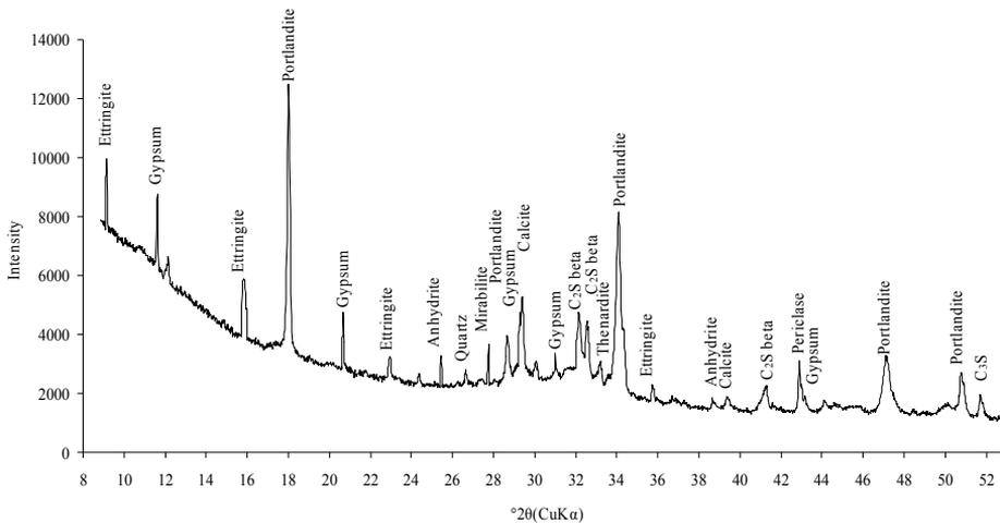
Figure 5.1.6 XRD analysis of CEM I paste after exposure to the 4.4 %  $\text{Na}_2\text{SO}_4$  solution for 91 days
