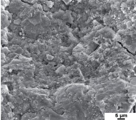
Figure 5.4.5 CEM III/A (60 % S) mortar stored for 91 days in the 4.4 %  $\text{Na}_2\text{SO}_4$  solution. Dense, but uneven micro-structure, and no needle-shaped ettringite nor plated-shaped  $\text{Ca}(\text{OH})_2$  can be observed.
