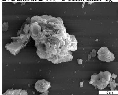
Figure 2.4.1 Shape of burnt shale particles (Raado and Nurm 2007).
