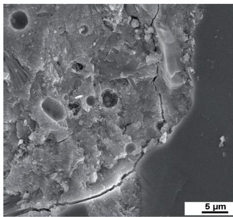
Figure 5.3.4 CEM II/A- $T_T$  (20%  $T_T$ ) mortar cured for 91 days in the saturated  $Ca(OH)_2$  solution. The cement stone is fragile, cracks.
