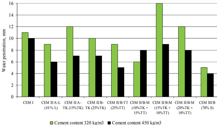
Figure 6.3.1 Water permeability of concrete by EVS-EN 12390-8 as the depth of penetration of water under pressure
