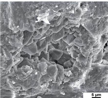
Figure 5.1.4 CEM I mortar after 91 days in the 4.4 % Na<sub>2</sub>SO<sub>4</sub> solution. Formation of gypsum crystals in an air void in near-surface region.
