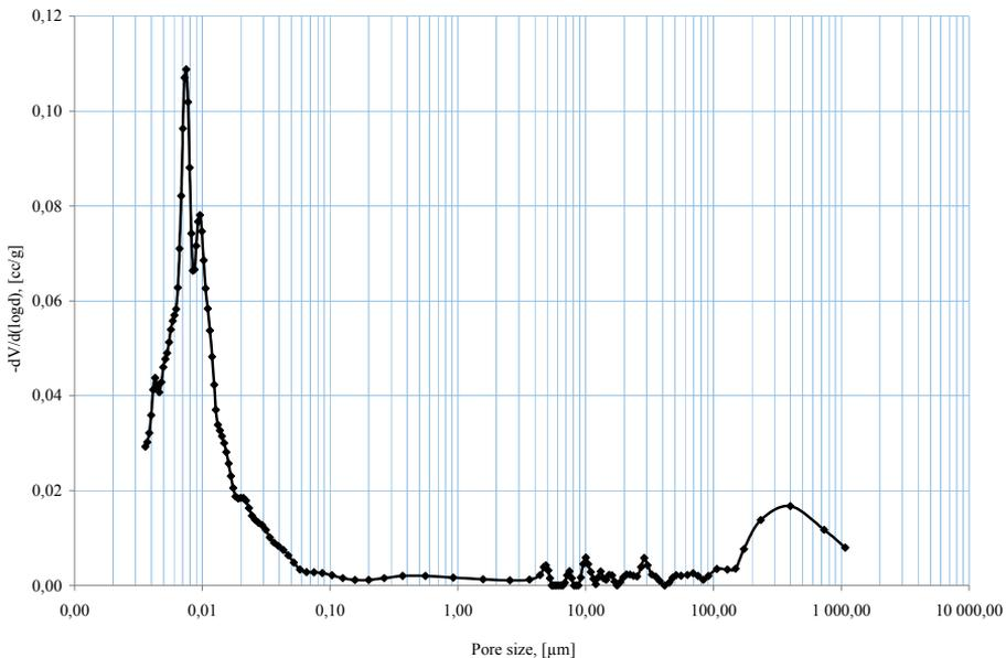
Figure 5.4.8 Pore size distribution of slag cement CEM III/A (60 % S) paste. Specimens were stored in the 4.4 %  $\text{Na}_2\text{SO}_4$  solution for 91 days
