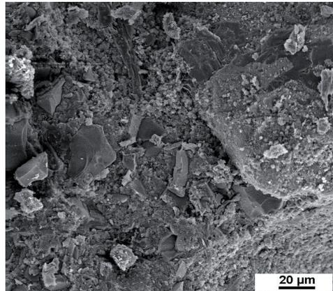
Figure 5.4.4 CEM III/A (60 % S) mortar cured for 14 days in the Ca(OH)<sub>2</sub> solution. Cement stone in the middle section of the specimen. Clearly distinguishable slag particles.
