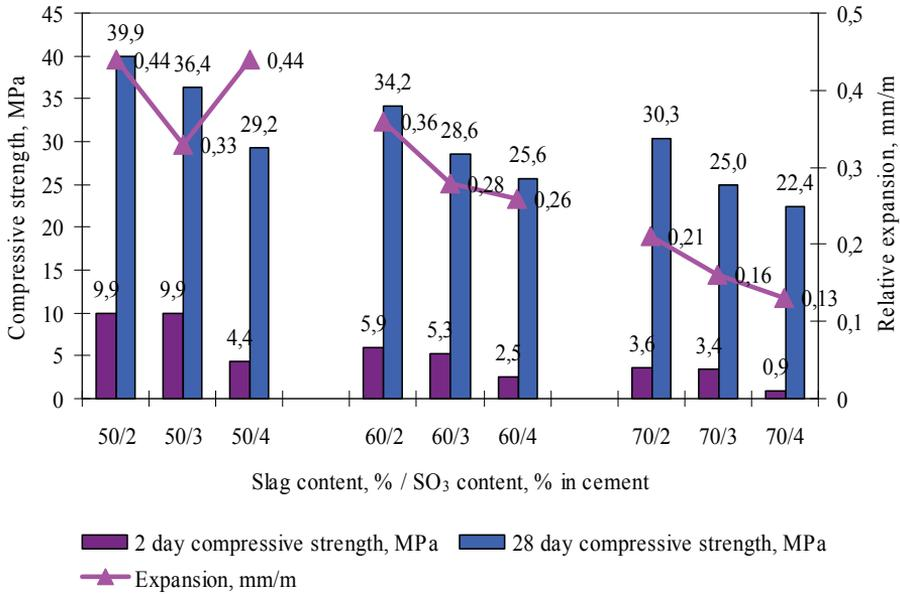
Figure 5.4.2 Influence of SO<sub>3</sub> level in slag cements for sulfate resistance and strength properties
