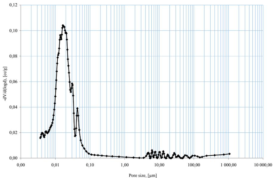
Figure 5.3.16 Pore size distribution of Portland burnt shale  $T_K$  cement CEM II/A- $T_K$  (20 %  $T_K$ ) paste. Specimens were stored in the 4.4 %  $Na_2SO_4$  solution for 91 days
