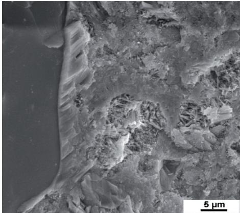
Figure 5.2.4 CEM II/A-L (10% L) mortar stored for 91 days in the 4.4 %  $\text{Na}_2\text{SO}_4$  solution. The main hydration products are C-S-H gel and needle-shaped ettringite in pores and voids.
