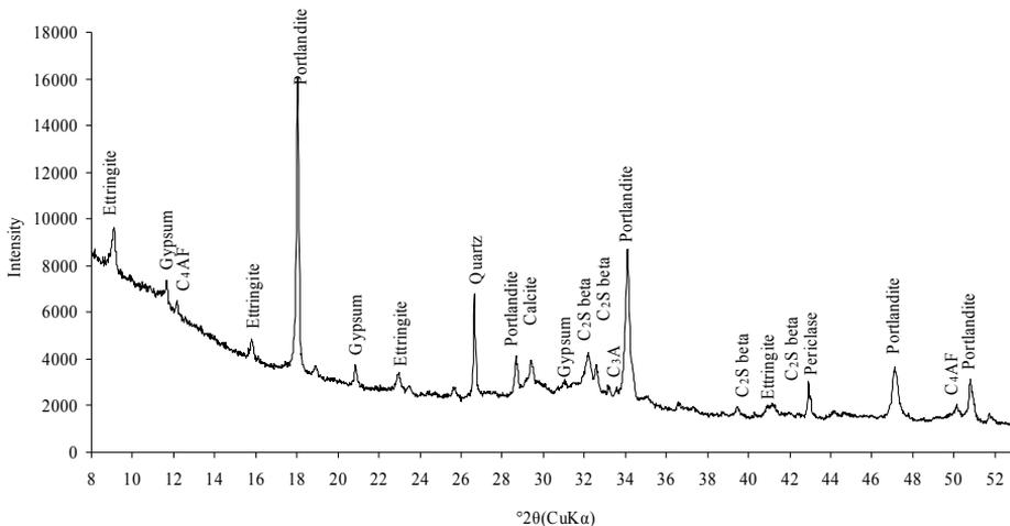
Figure 5.3.15 XRD analysis of Portland burnt shale T<sub>K</sub> cement CEM II/A-T<sub>K</sub> (20% T<sub>K</sub>) paste after exposure to the 4.4 % Na<sub>2</sub>SO<sub>4</sub> solution for 91 days
