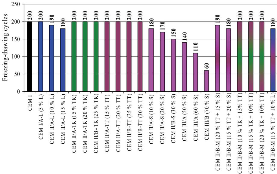
Figure 4.2.1 Frost resistance of cement mortar specimens
