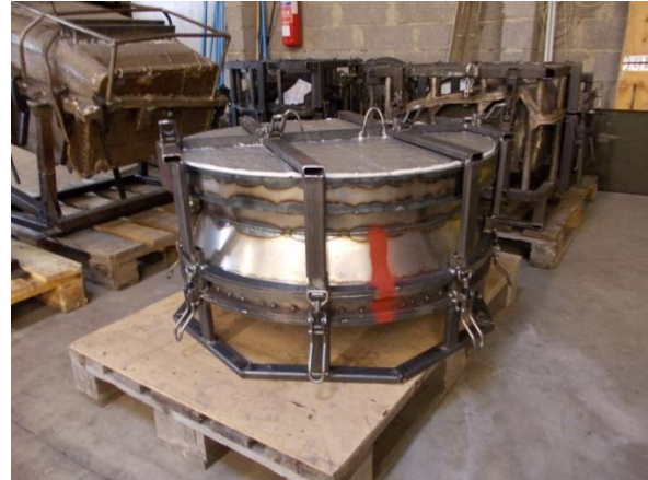
Figure 2.2 Rotational mold made of from steel sheet metal
