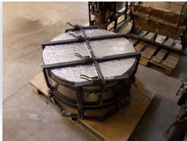
Figure 3.30 Rotational mold of the extension neck with heat reflective insulation material visible
