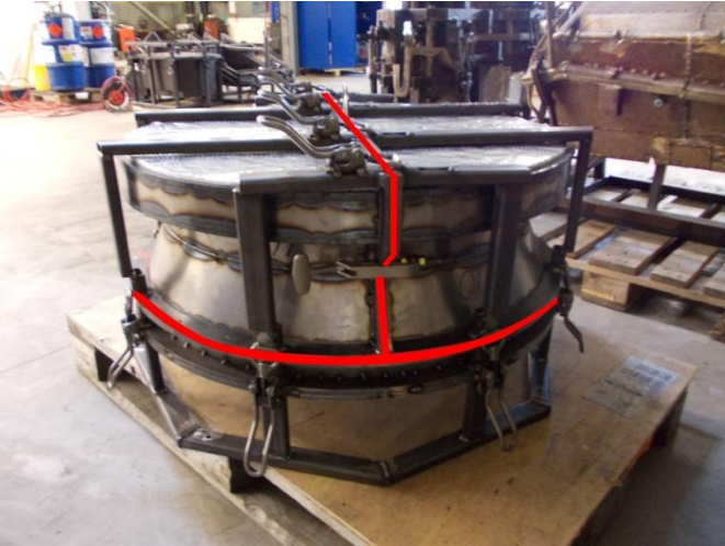
Figure 2.3 Sheetmetal three-part mold of an extension neck for a wastewater tank with 2 planar parting lines highlighted in red
