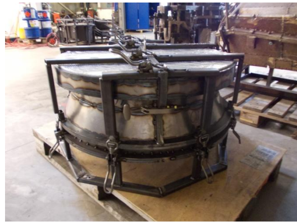
Figure 3.41 The finished rotational mold of the septic tank extension neck
