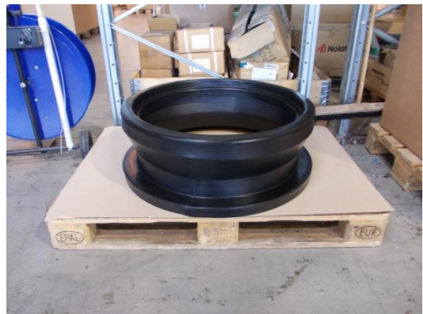
Figure 3.43 The finished septic tank extension neck
