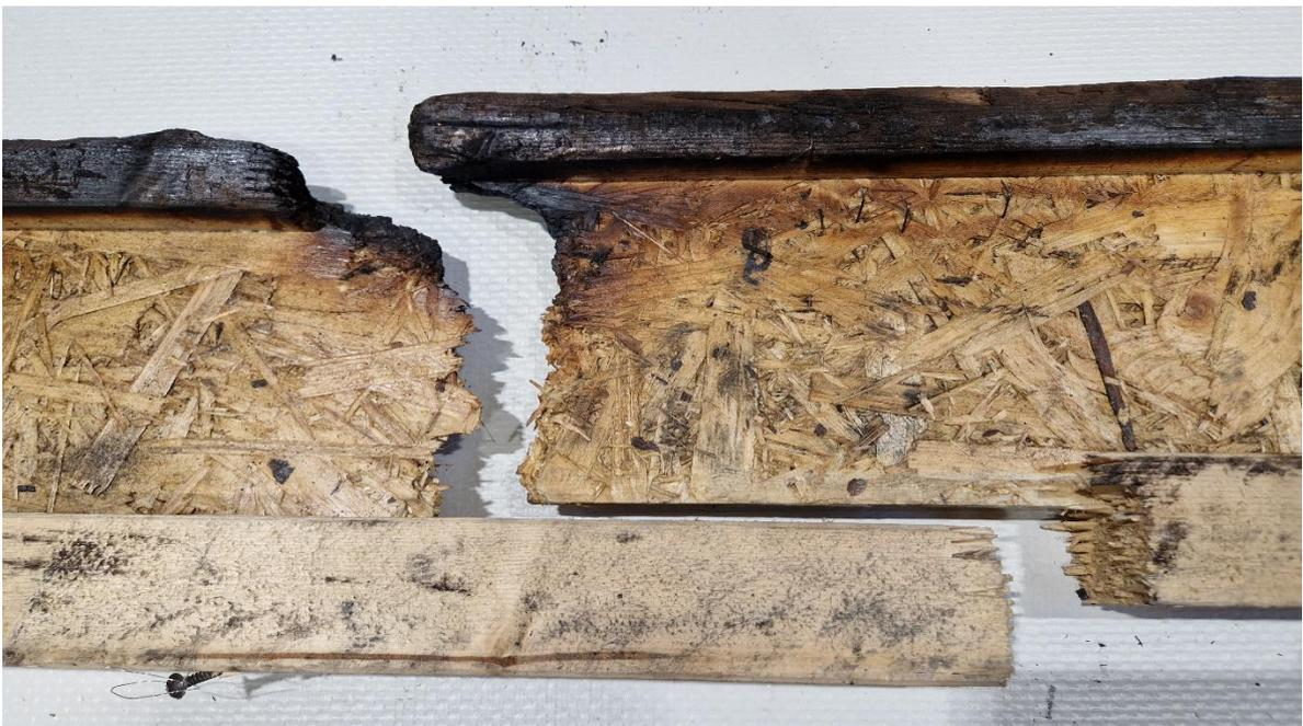
*Figure 4.2. Broken I-joist 2.4, position where the wood breakage took place.*
