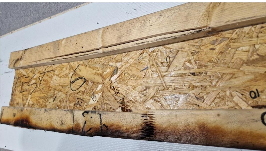
*Figure 5.2. Adhesive failure of a I-joist flange in the example of beam 4.3.*
