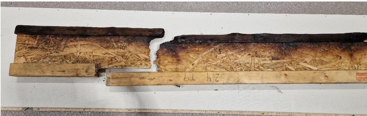
*Figure 4.1. Broken I-joist 2.4 in full length.*
