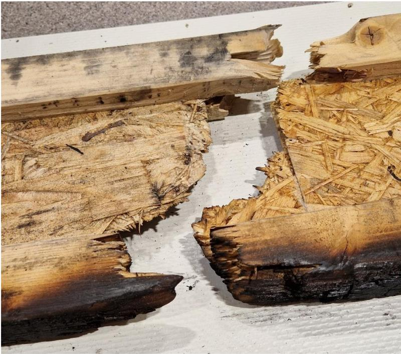
*Figure 5.1. Failure due to reaching the bearing capacity in the example of beam 2.2.*
