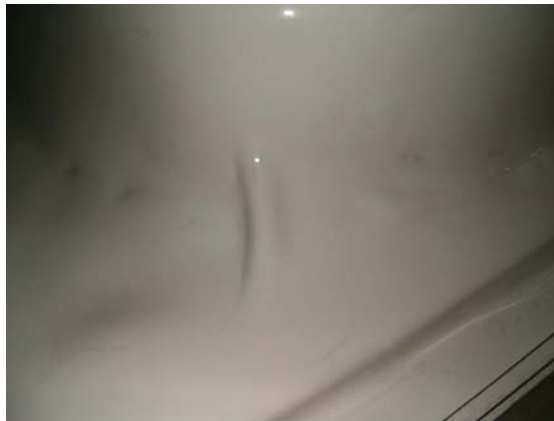
Figure 3.7. The ABS plastic part is too warm and vacuum doesn't work correctly
