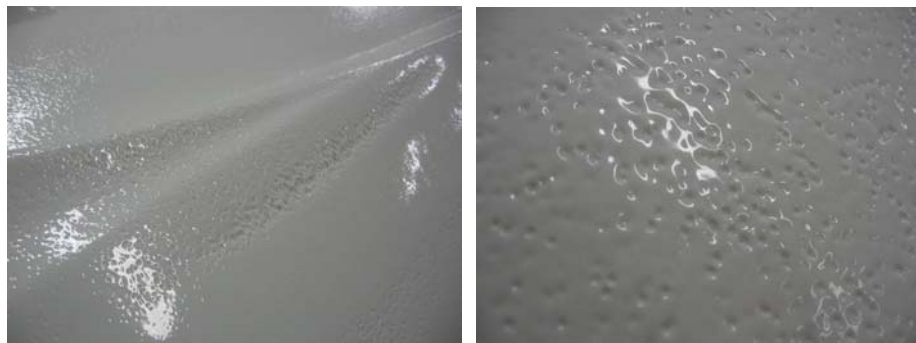
Figure 3.5. ABS sheet was wet before thermoforming (a) and zoom in picture (b)
