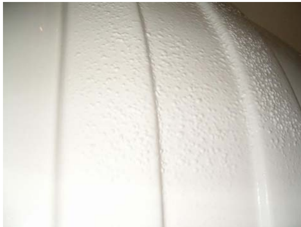
Figure 3.4. Surface defects – the ABS was wet before thermoforming
