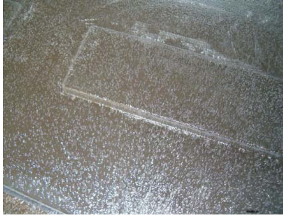
Figure 3.6. Surface defects – the polycarbonate was wet before thermoforming
