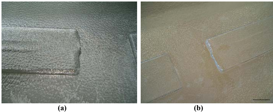
Figure 3.10. Critical outside radius - bubble (a) and hollow (b) of the wall
