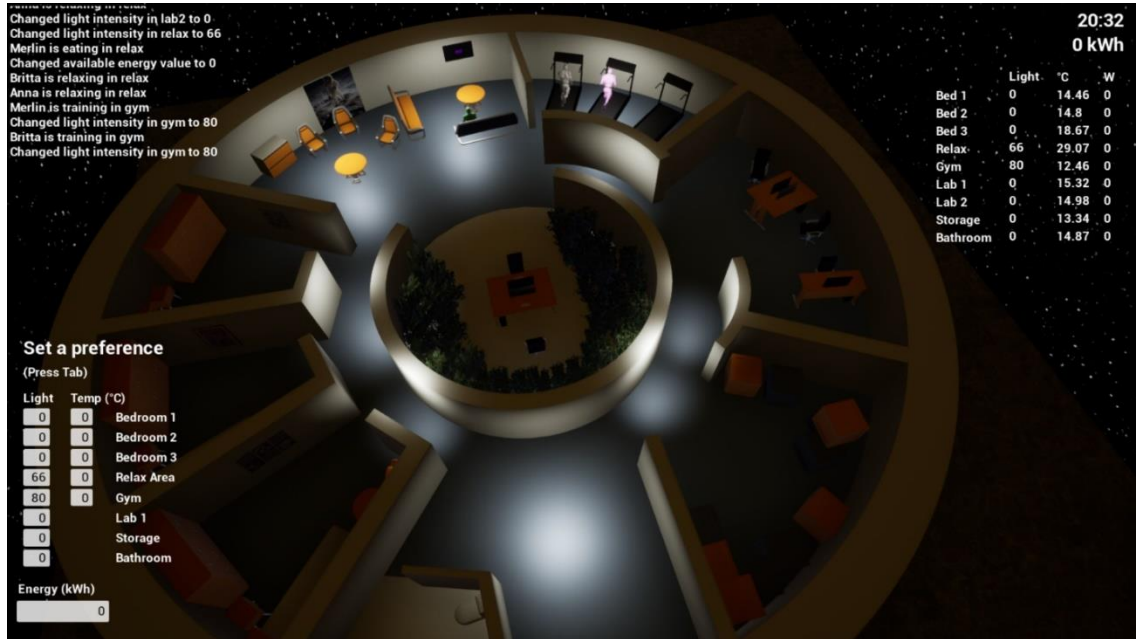
Figure 21. Changing the available energy to 0 makes all the power inputs go to 0 as well
