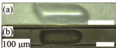
Fig. 4. Comparison of droplets using LED light. The results are recorded using (a) Raspberry Pi V2 camera running at 665 fps and (b) Basler Ace camera running at 750 fps. A flow rate of 4 \mu\text{L}/\text{min} for water and 8 \mu\text{L}/\text{min} for oil were used.
