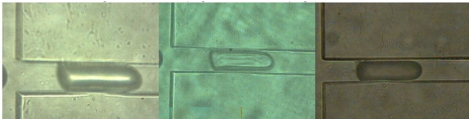
Figure 27. Images of droplets used for MATLAB PIQE function analysis. The results from left to right are 8.9607, 30.9641, and 8.9607 for Raspberry Pi V2, Raspberry Pi HQ, and Basler Ace cameras respectively, where smaller number indicates better image quality.
