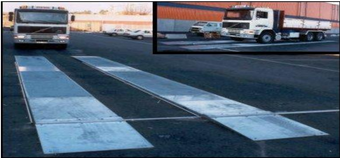
Figure 3.2. Concept of plate braking testing system [4]
