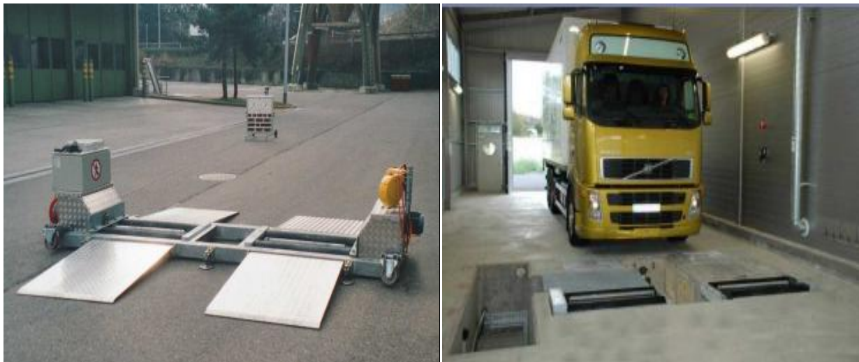
Figure 3.1. Roller tester for braking efficiency measurement concept [3].
