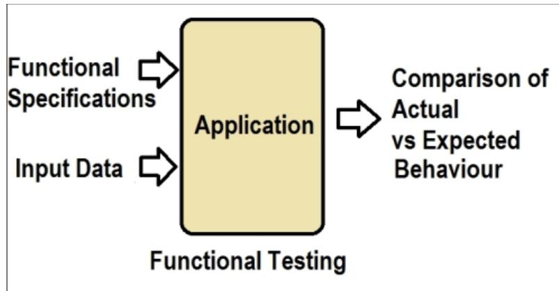
Figure 5. Functional testing architecture
