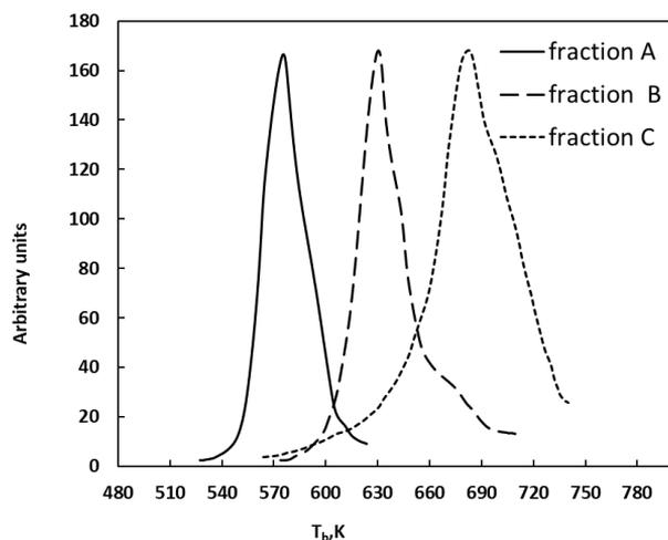
Figure 2.2 Indicative atmospheric boiling distributions (normalized by mass) for middle oil simple distillation cuts distilled under vacuum conditions (Figure 1, Paper III)
