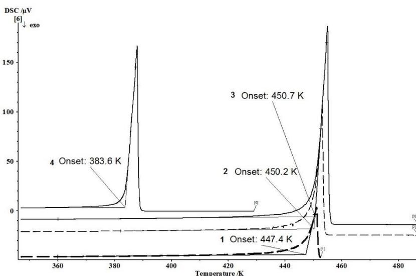
Figure 2.4 Boiling endotherms of toluene at around 101 kPa and at 500 kPa using different sample amounts (same as Figure 3, *Paper I*)
