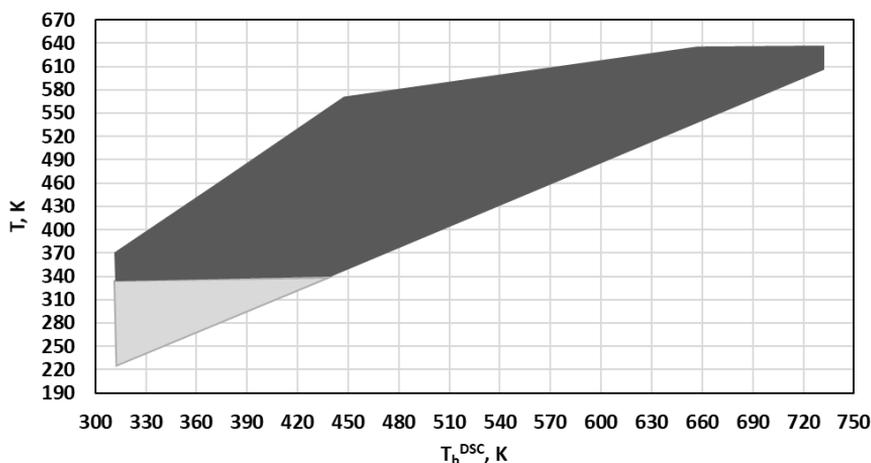
Figure 3.2 Tentative temperature ranges of the DSC method. Light grey triangle indicates temperature region where cooling is needed.
