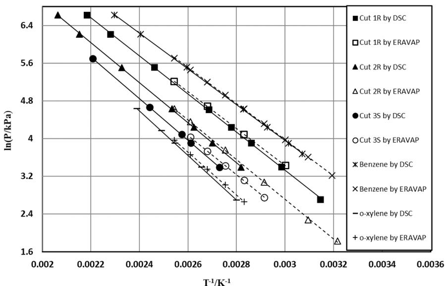
Figure 3.1 Vapor pressure data using DSC and ERAVAP. Solid lines present trendlines for DSC measurements and dashed lines for ERAVAP (same as Figure 4, Paper II)
