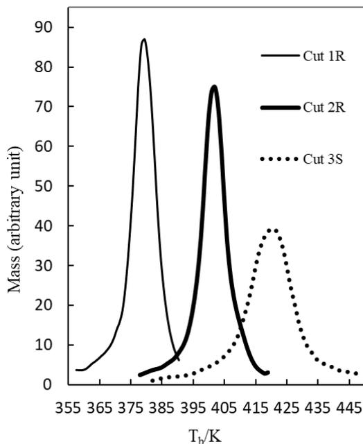
Figure 2.1 Indicative atmospheric pressure boiling point distributions (normalized for the same mass) for rectification and simple distillation cuts, distilled under atmospheric pressure (same as Figure 2, Paper II)
