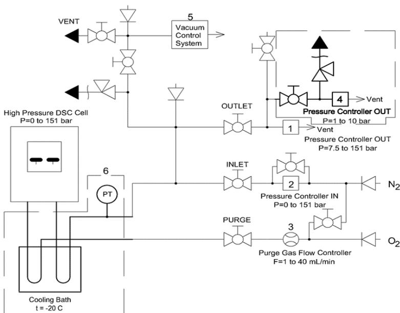
Figure 2.3. The scheme of the modified DSC equipment
