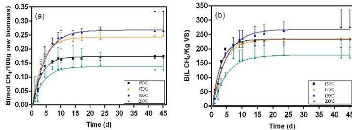
**Figure 7.** Biochemical methane results and respective fitting curves for samples from the liquid fraction of post-pretreatment broth pretreated at different temperatures (150 °C, 170 °C, 190 °C, and 200 °C). (a) results in mol CH<sub>4</sub>/100 g raw biomass; (b) results in L CH<sub>4</sub>/Kg VS.
