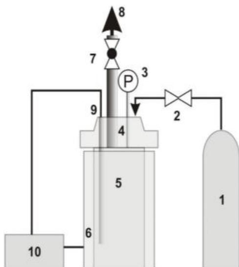
**Figure 4.** Diagram of Nitrogen explosive decompression pretreatment system. 1- N<sub>2</sub> tank, 2- pressure control valve; 3- manometer; 4- modified pressure vessel lid; 5- Parr instruments pressure vessel; 6- ceramic contact heater; 7- pressure release valve; 8- ventilation system; 9- thermocouple; 10- temperature controller unit [66]
