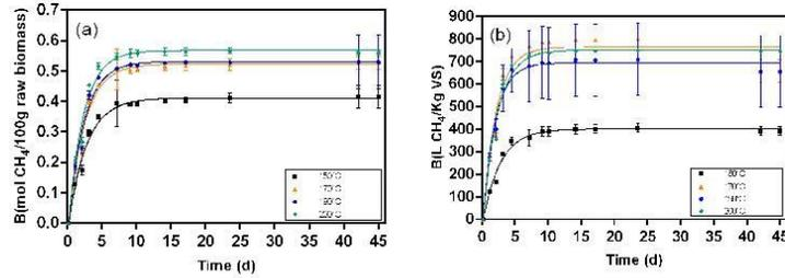
Figure 8. Biochemical methane results and respective fitting curves for samples from the liquid fraction post-hydrolysis broth pretreated at different temperatures (150 °C, 170 °C, 190 °C, and 200 °C). (a) results in mol CH<sub>4</sub>/100 g raw biomass; (b) results in L CH<sub>4</sub>/Kg VS.
