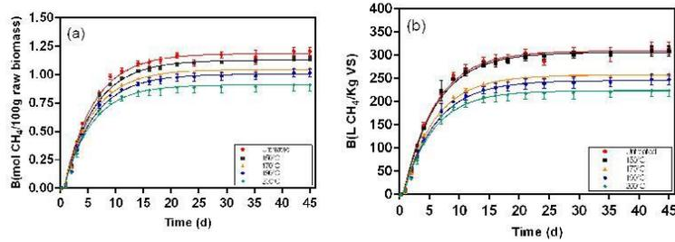
**Figure 5.** Biochemical methane results and respective fitting curves for samples from the solid fraction of post-pretreatment broth pretreated at 150 °C, 170 °C, 190 °C, and 200 °C. (a) results in mol CH<sub>4</sub>/100 g raw biomass; (b) results in L CH<sub>4</sub>/Kg VS.
