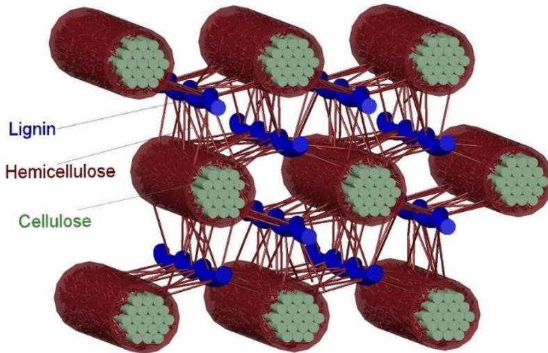
**Figure 2.** schematics of lignocellulosic biomass cells [33]
