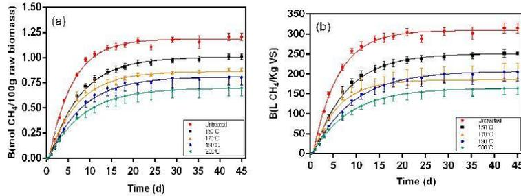
**Figure 6.** Biochemical methane results and respective fitting curves for samples from solid fraction of post-hydrolysis broth pretreated at 150 °C, 170 °C, 190 °C, and 200 °C. (a) results in mol CH<sub>4</sub>/100 g raw biomass; (b) results in L CH<sub>4</sub>/Kg VS.
