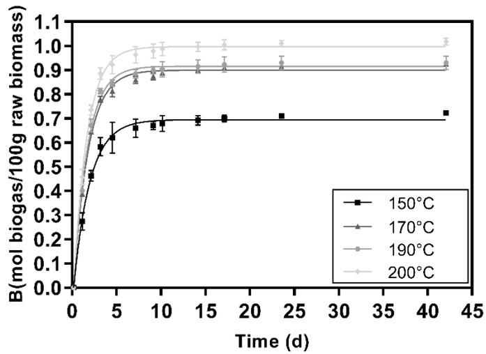
**Figure 8.** Liquid fraction after hydrolysis at 150 °C, 170 °C, 190 °C, and 200 °C in mol CH<sub>4</sub>/100 g raw biomass
