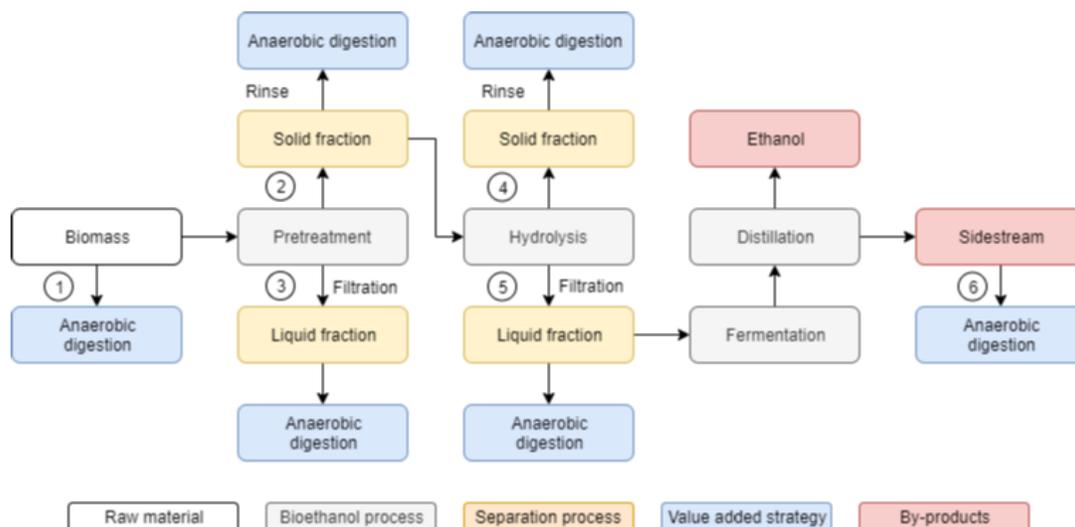
**Figure 1.** The production pathways utilized for this study to evaluate the potential of Napier grass (*Pennisetum purpureum/ elephant grass*) for biogas and bioethanol production by means of solid–liquid separation. 1—untreated Napier grass; 2—solid fraction of post-pretreatment broth; 3—liquid fraction of post-pretreatment broth; 4—solid fraction of post-hydrolysis broth; 5—liquid fraction of post-hydrolysis broth; 6— liquid samples of the post-distillation broth [23]
