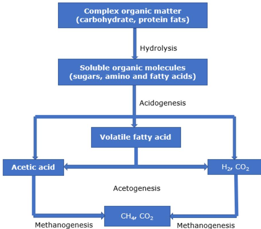
**Figure 3.** The three anaerobic digestion stages [93]
