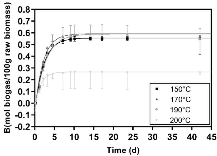
**Figure 9.** Liquid fraction after distillation at 150 °C, 170 °C, 190 °C, and 200 °C in mol CH<sub>4</sub>/100 g raw biomass
