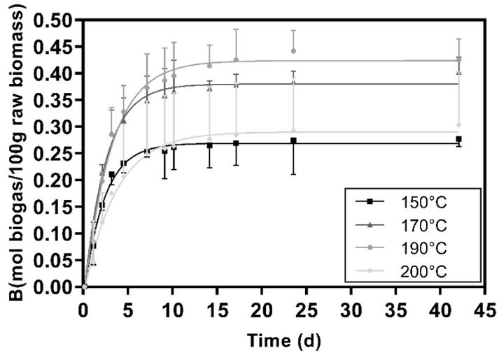
**Figure 7.** Liquid fraction after pretreatment at 150 °C, 170 °C, 190 °C, and 200 °C in mol CH<sub>4</sub>/100 g raw biomass
