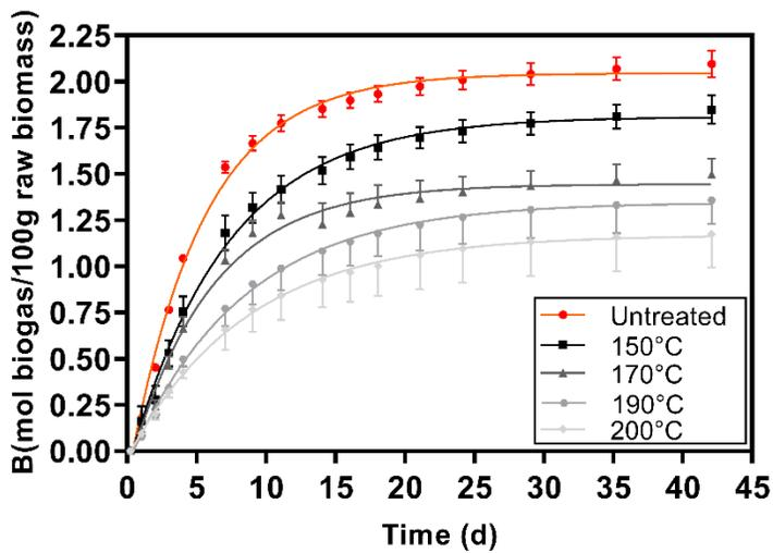
**Figure 6.** Solid fraction after hydrolysis at 150 °C, 170 °C, 190 °C, and 200 °C in mol CH<sub>4</sub>/100 g raw biomass
