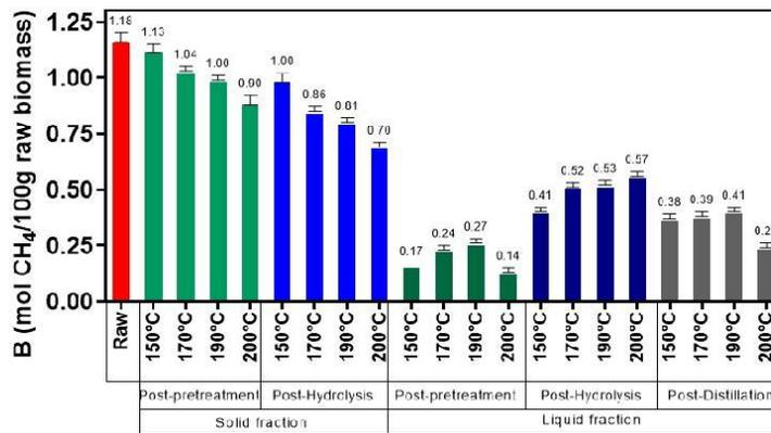
Figure 10. Maximum methane yield (B<sub>max</sub>) of the fitting curves of samples from the solid and liquid fractions.
