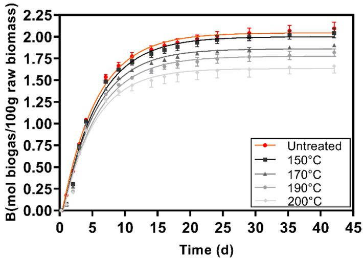
**Figure 5.** Solid fraction after pretreatment at 150 °C, 170 °C, 190 °C, and 200 °C in mol CH<sub>4</sub>/100 g raw biomass
