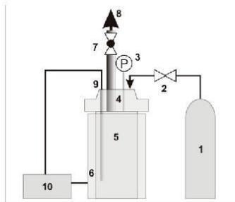
**Figure 1.** Schematic diagram of the 2 L pressure vessel system (series 4600) for NED pretreatment: 1—nitrogen tank; 2—pressure control valve; 3—manometer; 4—modified pressure vessel cap; 5—Parr instruments pressure vessel; 6—ceramic contact heater; 7—pressure release valve; 8—ventilation system; 9—thermocouple; 10—temperature controller unit [28].
