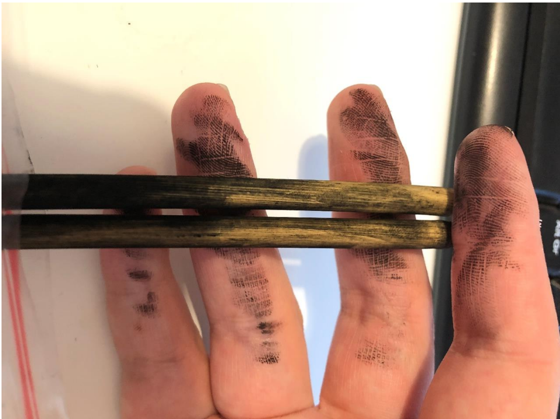
Figure A.6 Straws without pre-treatment, boiled with 1 tbs of PME Black liquid food colour for 18 min
