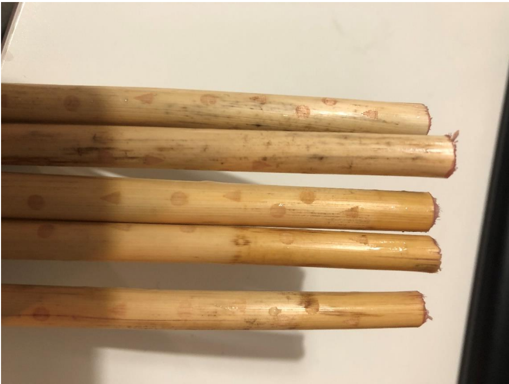
Figure B.11 Laser engraved straws with no pre-treatment inside cherry juice for 3 hours
