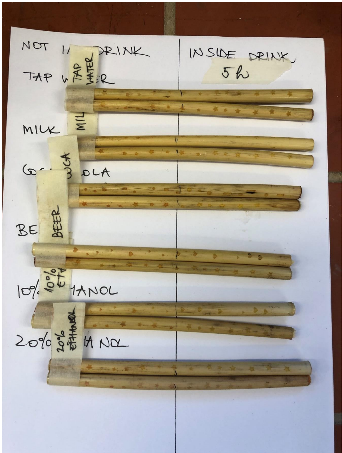
Figure C.16 Straws with PME Orange after 5x1 h drink test and 5x wash test (straws that are thermally modified before colour for 1 h at 100°C, colour oven dried for 1.5 h at 100°C)
