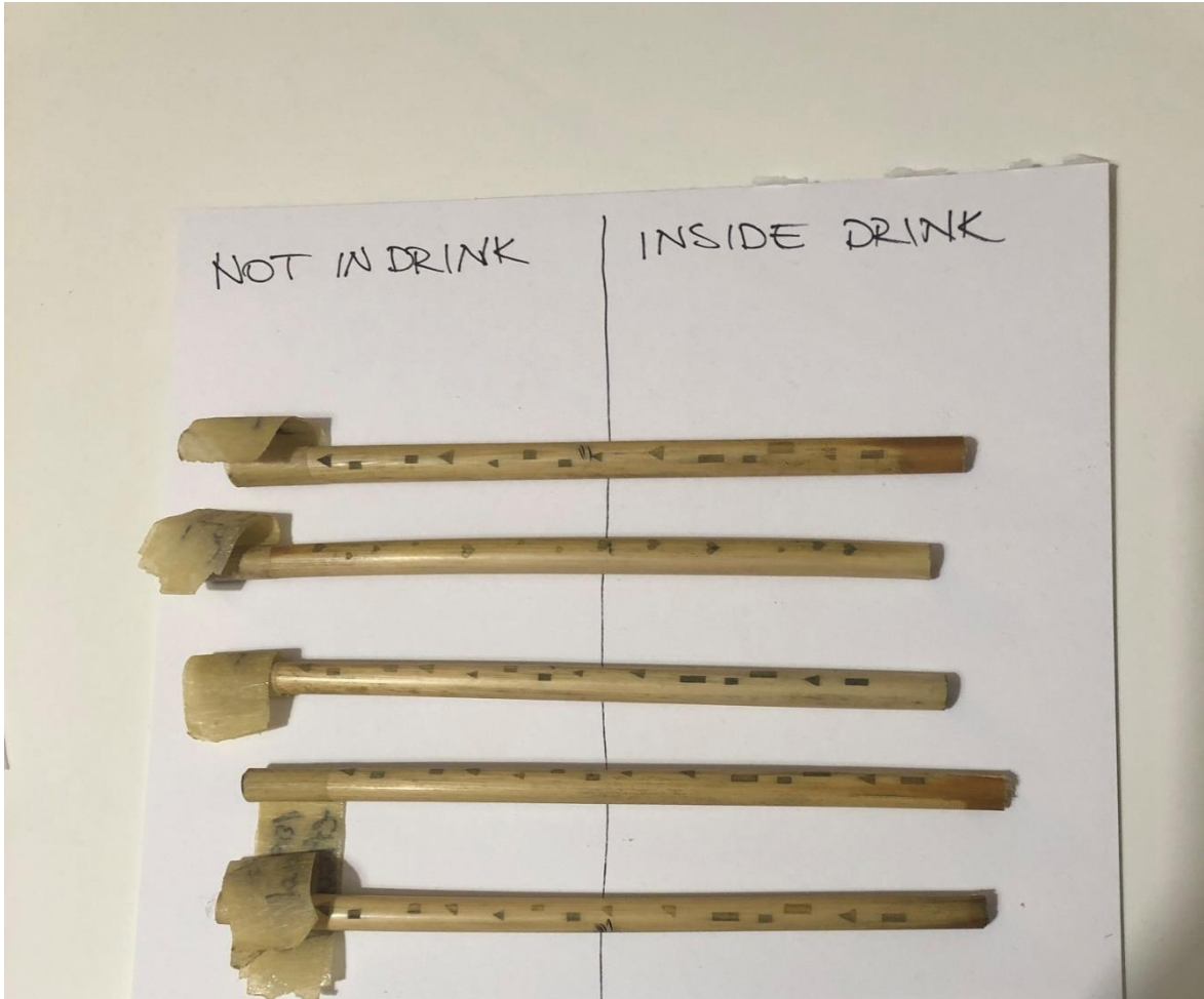
Figure C.17 Straws with PME Moss Green after 1x 1 h drink test and 24 extreme condition test inside water at 70°C for 24 hours (colour oven dried after the excess colour was removed with a paper napkin for 1.5 h at 100°C)
