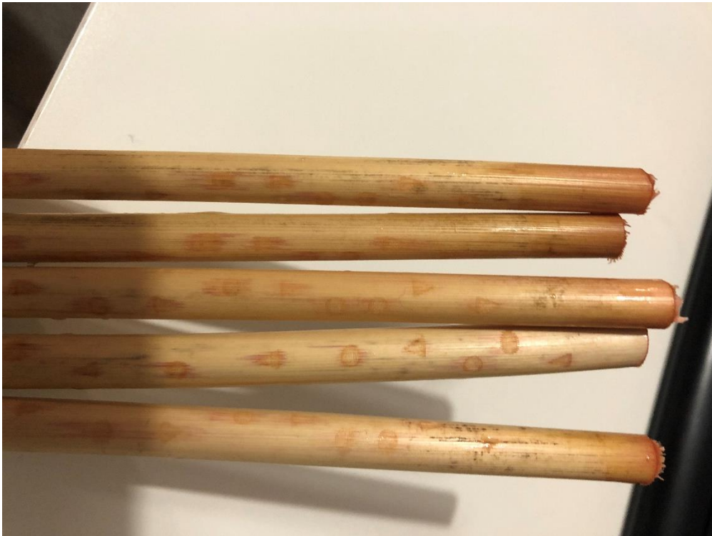
Figure B.10 Laser engraved straws with no pre-treatment inside beetroot juice for 3 hours
