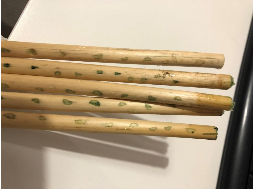
Figure B.12 Laser engraved straws with no pre-treatment covered with spirulina powder and a drop of water for 3 hours
