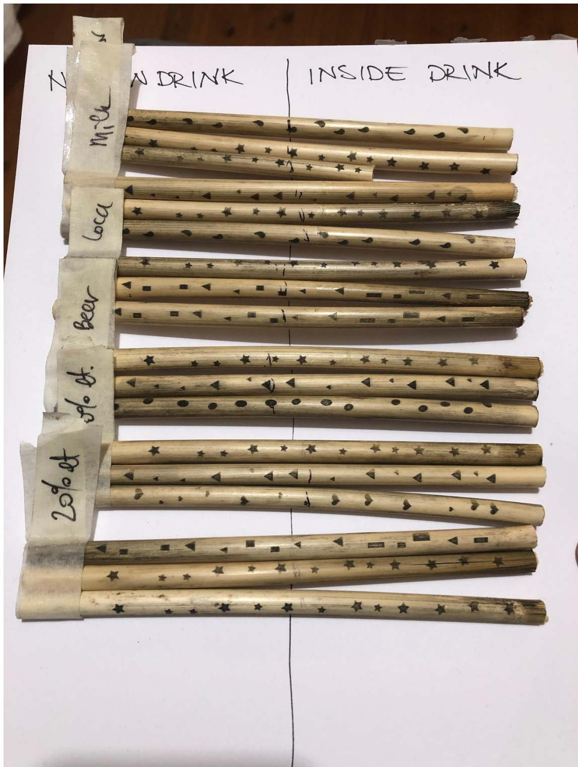
Figure 3.8 Straws with PME Black after 5x1 h drink test and 5x wash test (colour oven dried after the excess colour was removed with a paper napkin for 1.5 h at 100°C)
