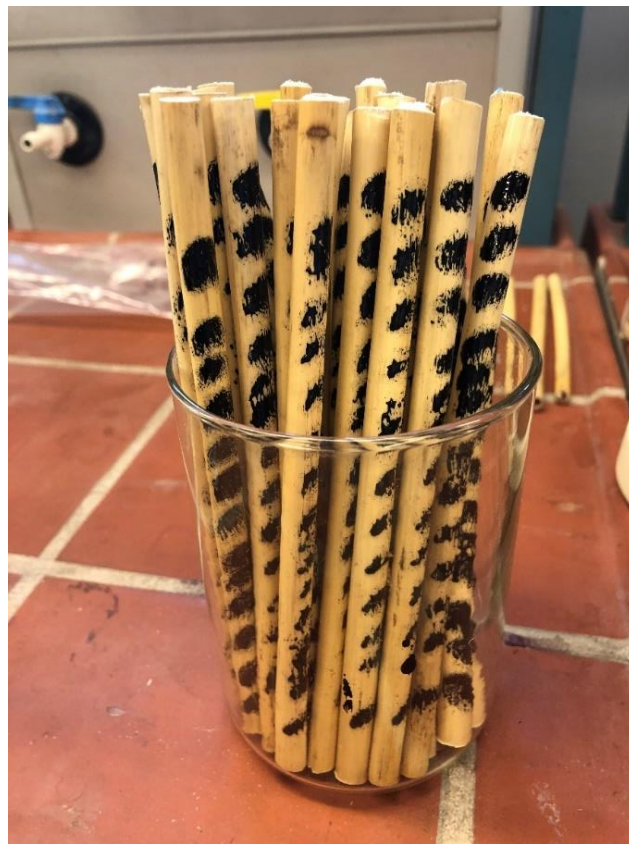
Figure 2.10 Laser engraved straws after colouring (excess colour on the straws)
