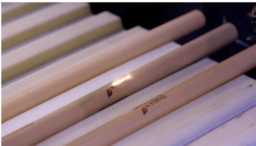
Figure 1.3 Laser engraving bamboo straws ("Alfexlaser," 2018)
