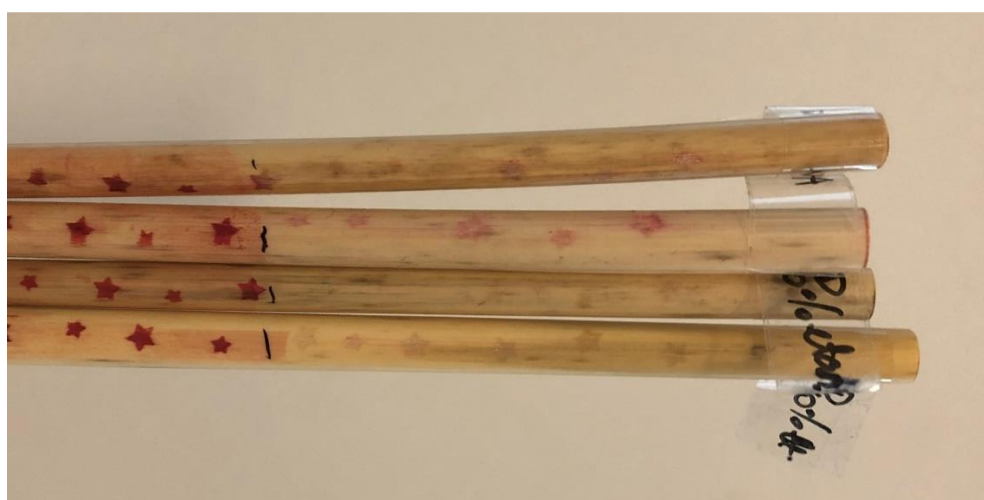
Figure 3.7 Laser engraved straws with Sugarflair Pink after 4 hours of durability testing
