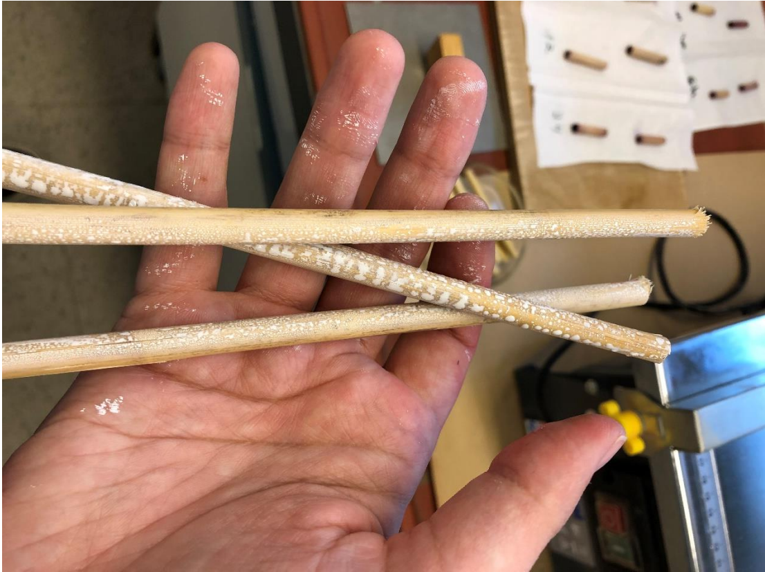
Figure A.5 Straws without pre-treatment, sprayed with 50/50 PME White paste/water solution with spray gun
