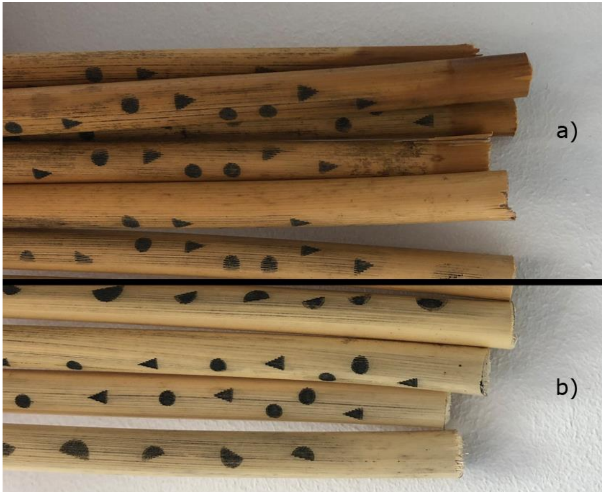
Figure 3.6 Coloured straws: (a) Oven dried at 160°C for 20 min; (b) Oven dried at 100°C for 1.5 h
