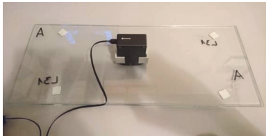
FIGURE 2. Measuring residual stresses with scattered light polariscope SCALP-05
